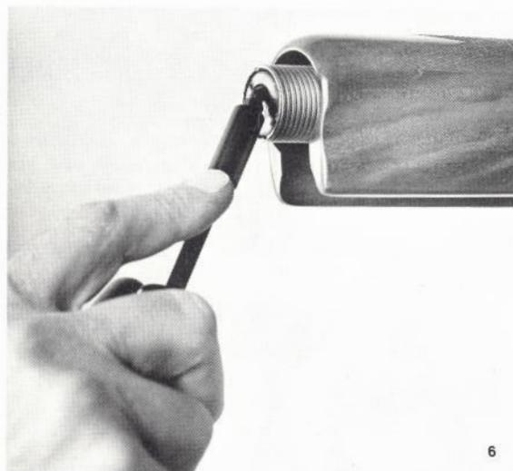
4. The plug is under spring compression and when the retainer ring is removed, plug will pop up.
