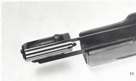
5. Now depress shell latch on ejection-port side of receiver and move forearm rearward completely to stop.
