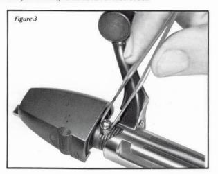
Note: In assembly, make sure that the threaded (back-end) portion of the firing pin is screwed-in flush with the rear surface of the cocking piece. If the flat on the firing pin (visible through hole in bolt sleeve) does not appear to be in alignment, unscrew the firing pin until alignment is correct. This method of re-assembly insures proper firing pin travel and protrusion.
