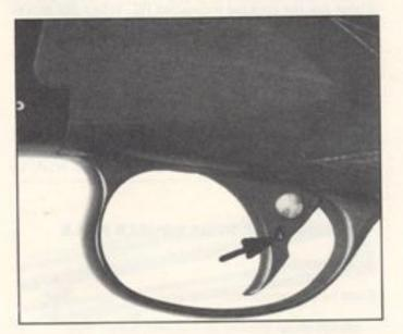
Remember that you press the selector button IN to choose which barrel fires first. By pulling the trigger [35] a second time, the other barrel will fire. NOTE: The finger must free the trigger between shots and be pulled again to fire the second barrel. The major advantage to this type of firing mechanism is that it is not recoil-operated. The second barrel will fire even if the first barrel is empty or misfired.
