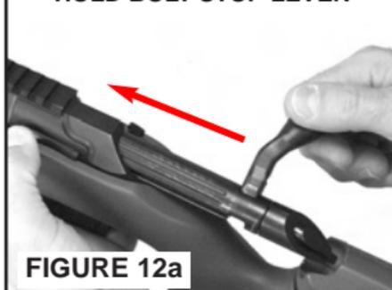
HOLD THE BOLT STOP IN - AS YOU ROTATE THE BOLT TO AVOID CATCHING THE BOLT STOP IN THE BOLT FLUTES
