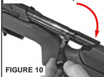
ROTATE BOLT HANDLE UNTIL BOLT STOP ENGAGES
