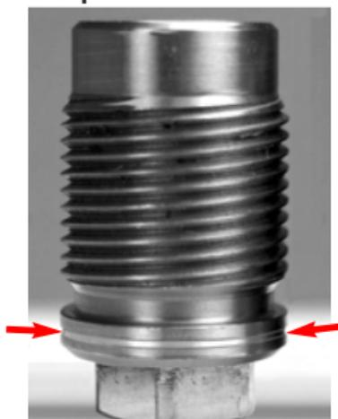
**NOTE :** This Breech Plug has an identifier groove shown here - at arrow.
