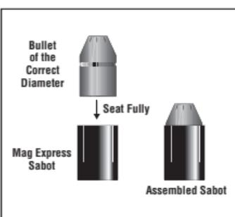
**The Assembled Sabot Must Be Seated Firmly On The Powder Charge.**
