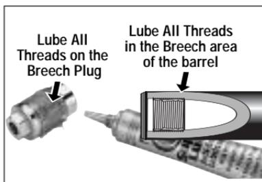
After your G2 Contender muzzleloader has been reassembled, check the hammer/trigger mechanism to ensure that there is no excess lubricant on any surface which could impede safe operation of the firearm.
