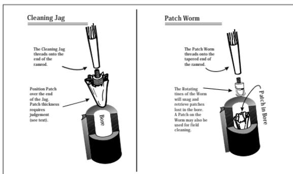
Thompson/Center does not package the worm with each firearm. This is an optional tool and must be purchased separately (one size fits all calibers - see current catalog). The worm is an extremely important muzzleloading tool and every shooter should carry one in his implement bag. While its prime purpose is to retrieve "lost patches", it can also be used for field cleaning. To do so you simply catch the cleaning patch on the tines of the worm and push it into the bore in the conventional manner.
