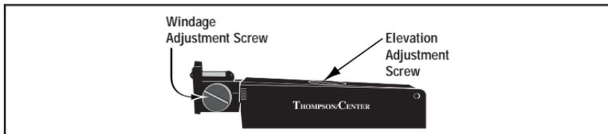
To adjust the windage it is necessary to move the entire rear sight leaf left or right by using the slotted screw head on the right side of the rear sight (as viewed from the receiver end of the sight). Move the rear sight blade in the direction you want your shots to hit - (Example; Turn the screw clockwise - thereby moving the sight blade to the right, to move your shots to the right and counter-clockwise to move the shots to the left).
