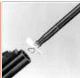
After removing all the fouling, follow up with a few dry patches to thoroughly dry the bore. If the gun is to be stored for any length of time, follow the dry patches up with a good protectant lubricant like T/C's All Natural Lube Bore Butter.
