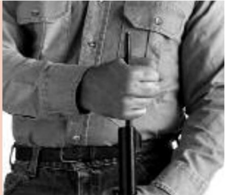
After the projectile is seated tightly against the charge, mark your ramrod to indicate the correct loaded depth of the powder plus the projectile (as shown below)
