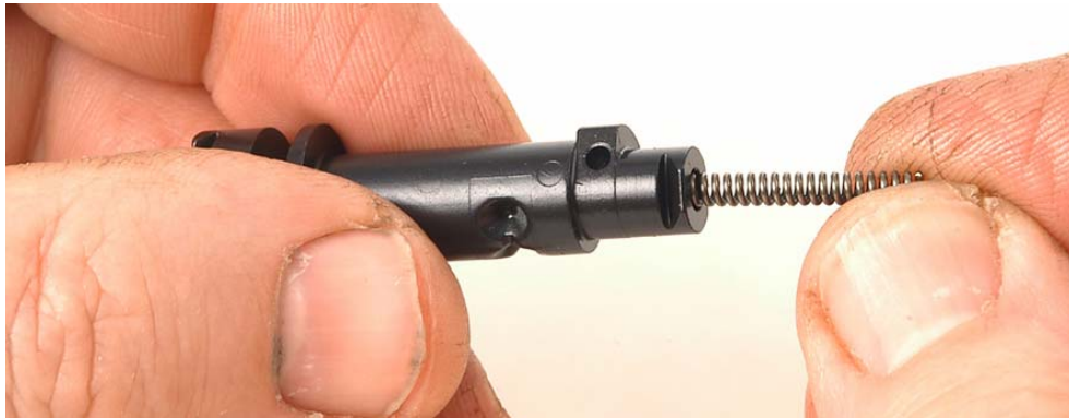
Figure 8-84. Inserting the Safety Left-Hand Plunger
