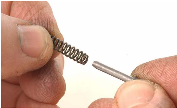
Figure 8-95. Assembling Sear Plunger Spring
