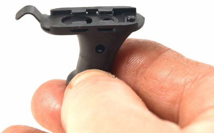
Figure 8-73. Cocking Handle Securing Spring
