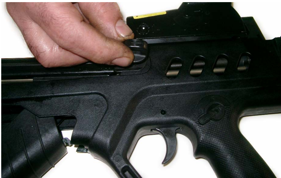
Figure 8-8. Inserting the Forward Sling Sleeve
