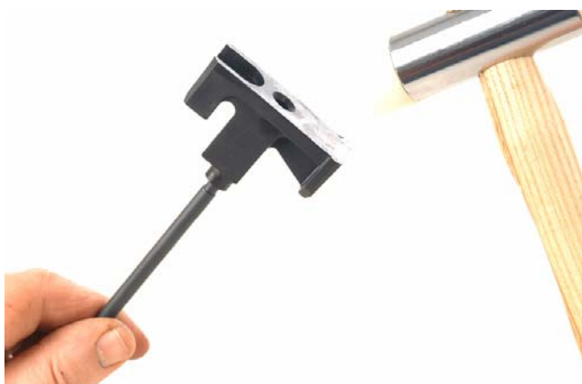
Figure 8-65. Securing the Bolt Carrier Guide Bar to the Buffer
