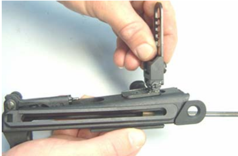
Figure 8-107. Assembling the Sight on the Cocking Handle Assembly
