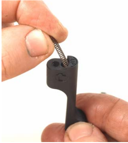
Figure 8-78. Inserting the Elevation Plunger Spring and Plunger
