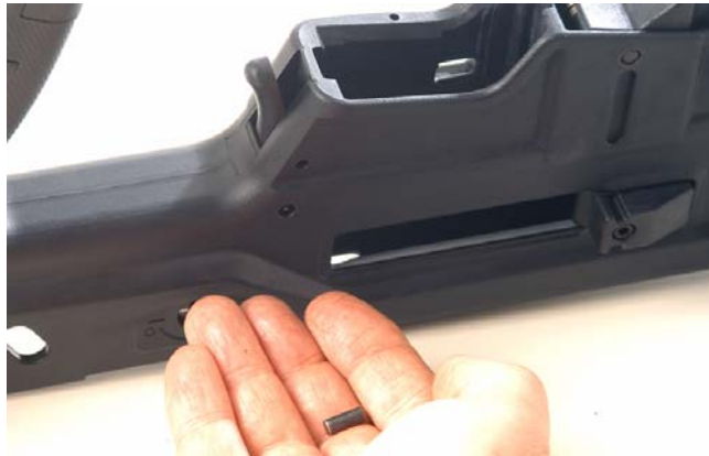
Figure 8-31. Installing the Magazine Release Lever Pivot
