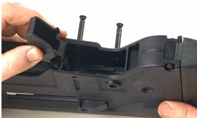
Figure 8-45. Installing the Bolt Carrier Stopper into the Receiver
