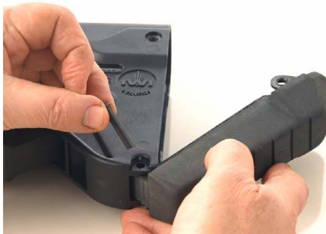
Figure 8-41. Inserting the Butt Pivot
