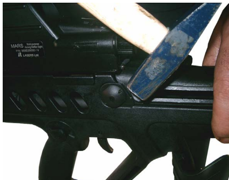
Figure 8-11. Inserting the Security Pin
