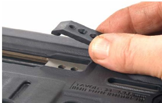
Figure 8-52. Installing the Ejection Port Shield
