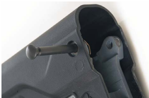
Figure 8-55. Installing the Butt Locking Pin
