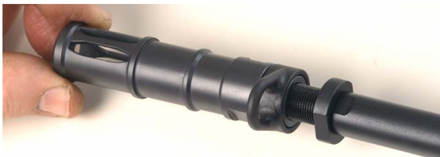
Figure 8-111. Screwing the Suppressor on the barrel
