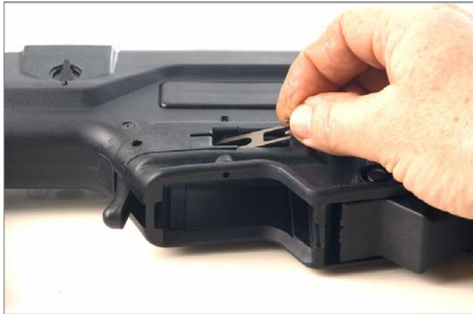
Figure 8-34. Installing the Magazine Connector Lever
