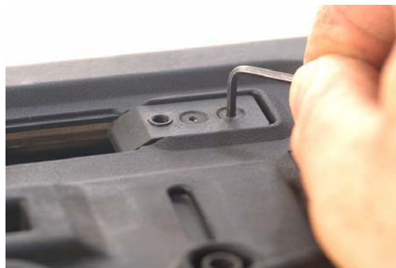
Figure 8-53. Securing the Ejection Port Shield
