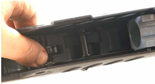
Figure 8-25. Trigger in Receiver
