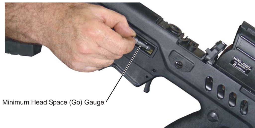
Figure 10-1. Minimum Head space Gauge Inspection
