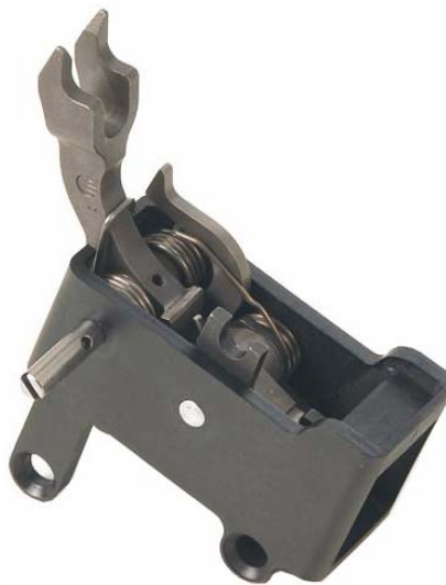
Figure 8-102. Inserting the Hammer Pivot
