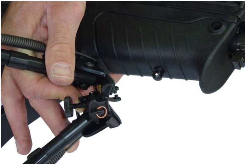
Figure 8-122. Removing the Bipod from the Rifle Grip
