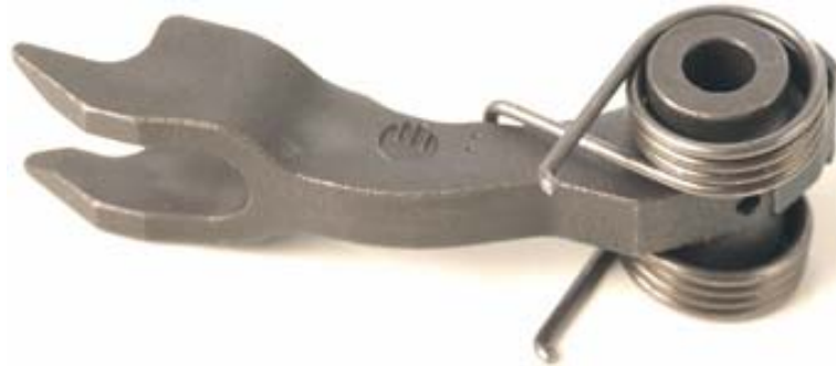
Figure 8-97. Assembling the Hammer and Hammer Spring
