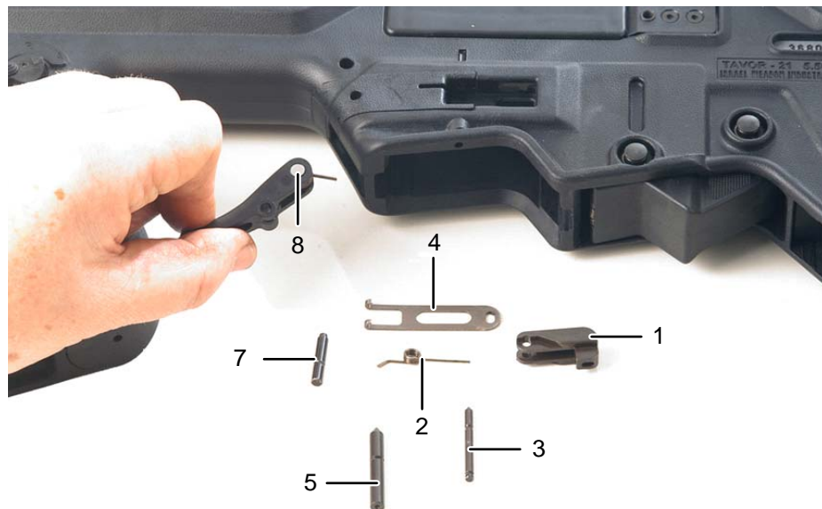
Figure 8-28. Installing the Magazine Release Lever Spring
