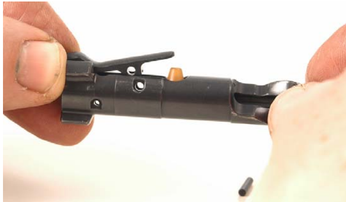
Figure 8-61. Inserting the Extractor Spring
