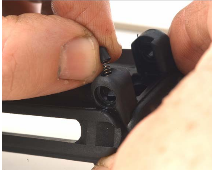
Figure 8-67. Inserting the Windage Screw Plunger
