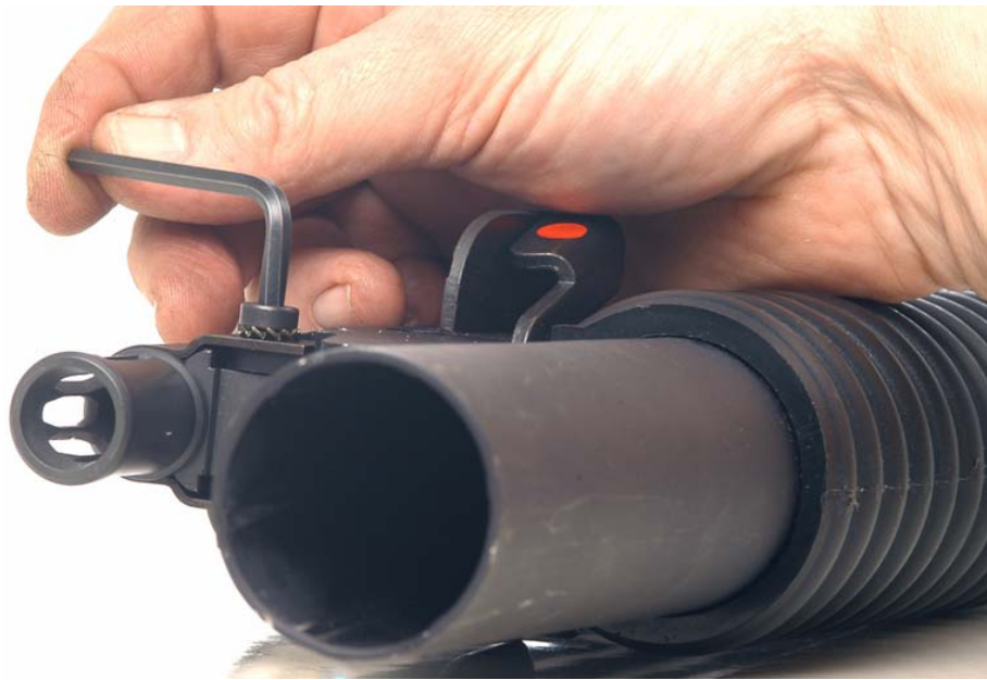
Figure 8-117. Installing the Cocking Handle Assembly
