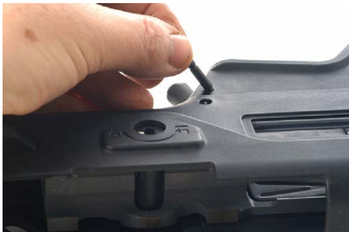
Figure 8-32. Installing the Connector Pin
