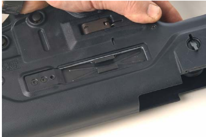
Figure 8-47. Inserting Ejection Port Cover Base
