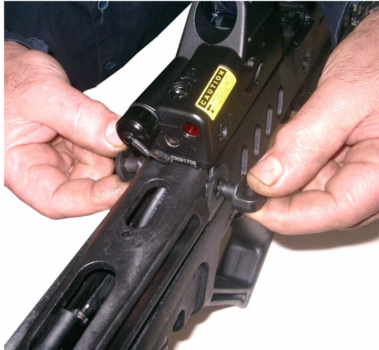
Figure 8-9. Screwing the Forward Sling Sleeve
