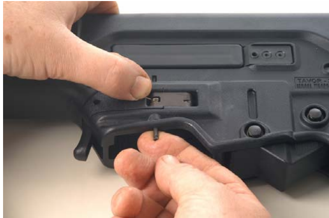
Figure 8-36. Installing the Magazine Catch Pin
