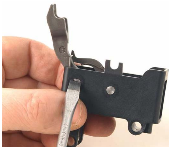
Figure 8-103. Locating the Hammer Pivot Hole
