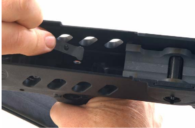
Figure 8-20. Inserting Safety Position Spring
