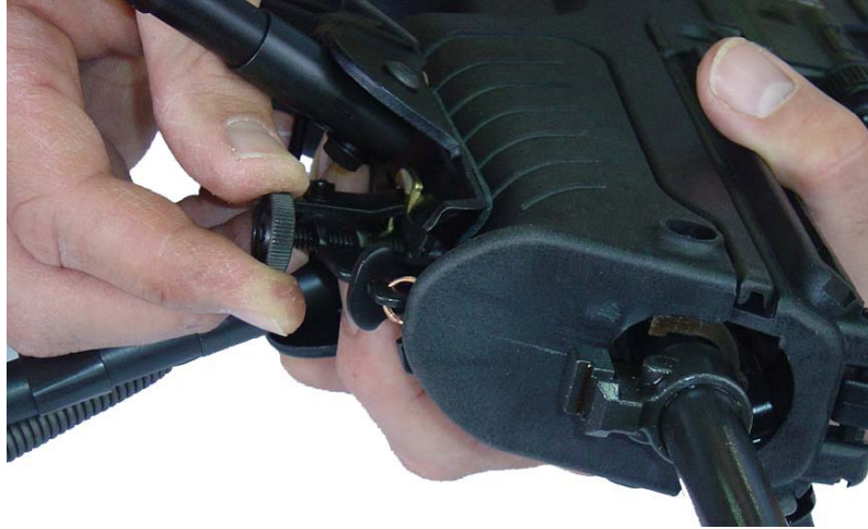
Figure 8-120. Releasing the Bipod Screw
