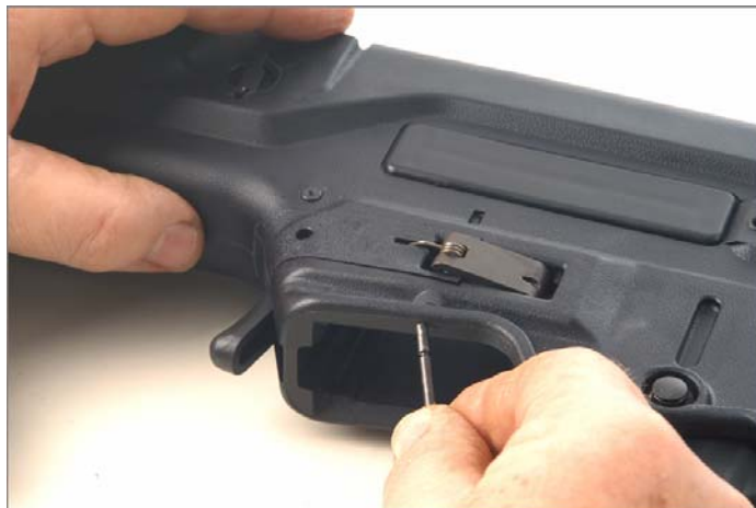
Figure 8-35. Installing the Magazine Catch
