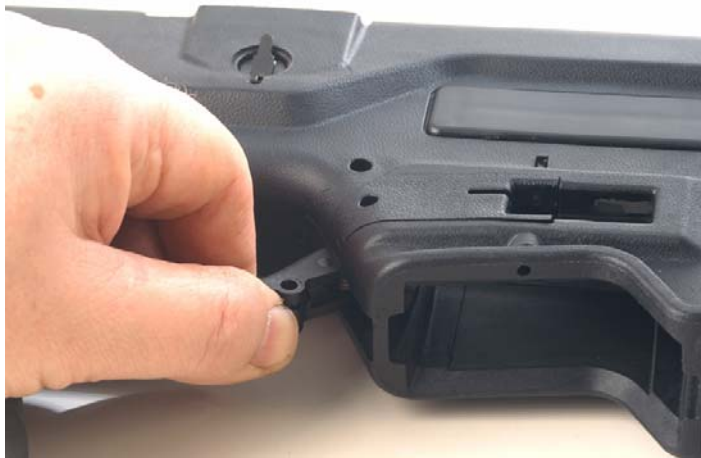
Figure 8-29. Installing the Lever into the Receiver
