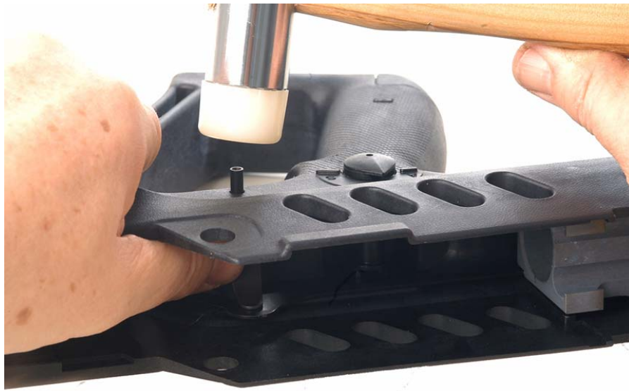
Figure 8-26. Inserting the Trigger Pin
