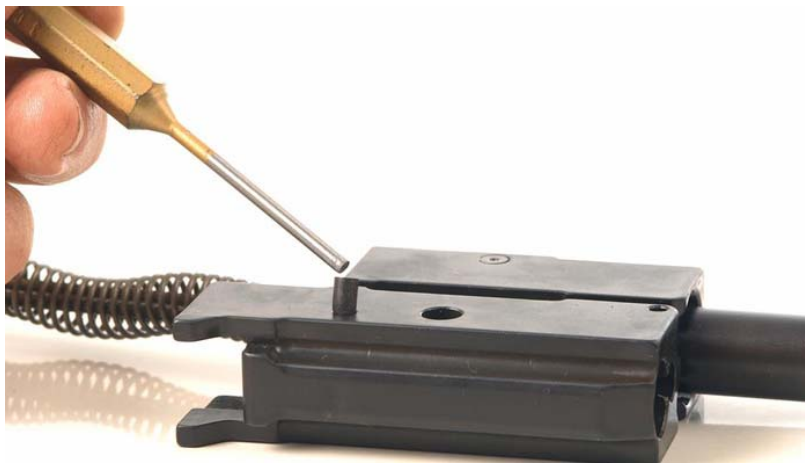
Figure 8-91. Inserting the Bolt Carrier Back Pin
