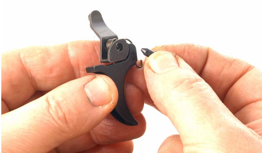
Figure 8-24. Inserting the Trigger Pin into the Trigger
