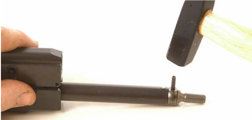
Figure 8-90. Inserting the Piston Connector Pin
