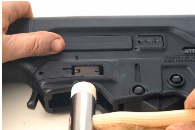
Figure 8-37. Securing the Magazine Catch Pin
