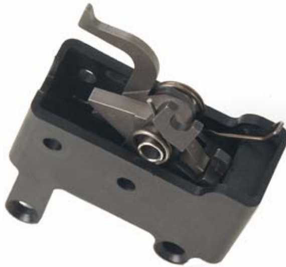
Figure 8-99. Assembling the Automatic Sear Spring
