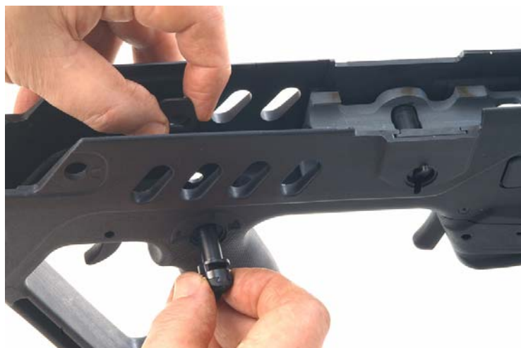
Figure 8-21. Inserting the Safety into Place
