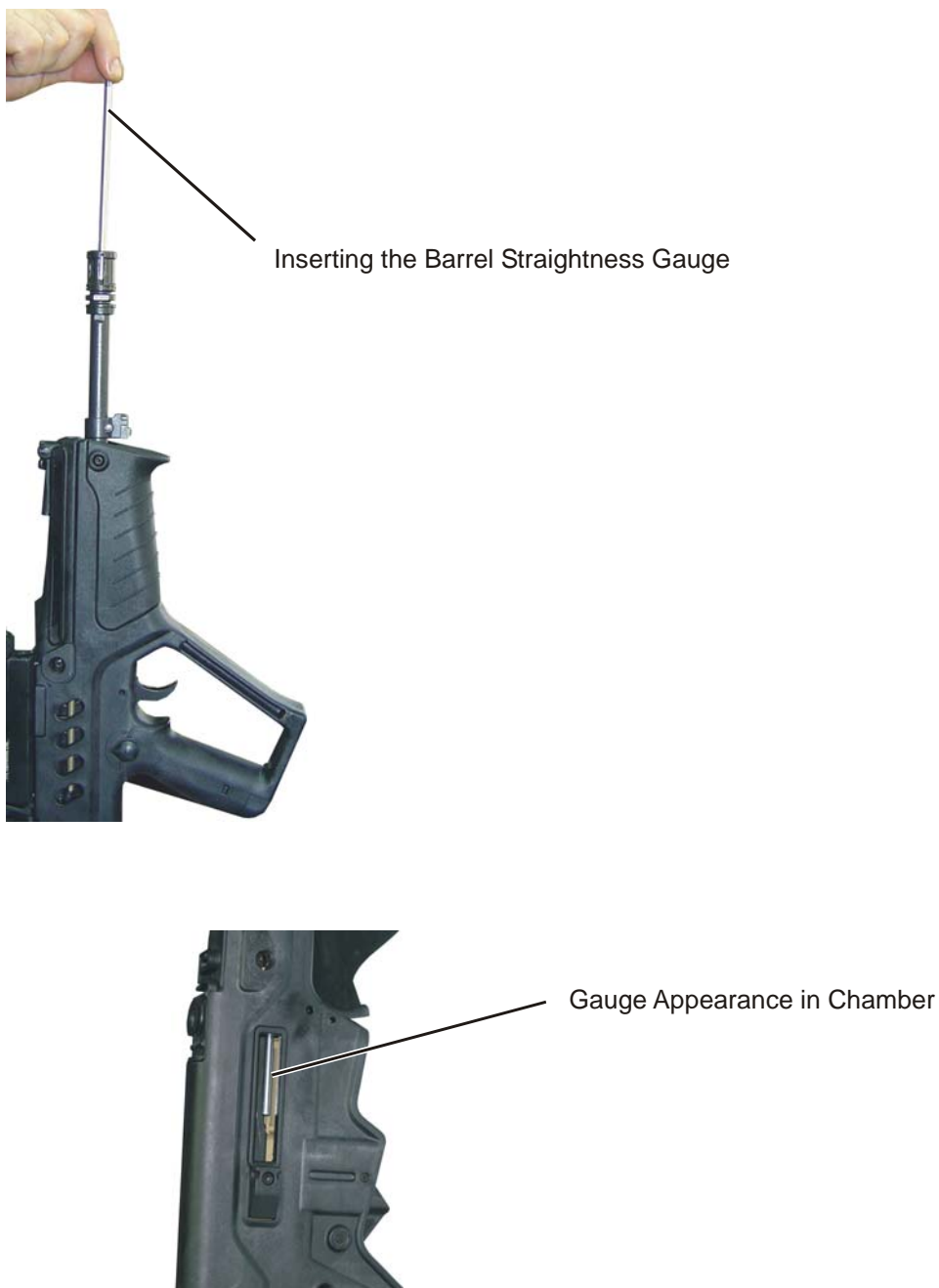
Figure 10-3. Barrel Straightness Inspection
