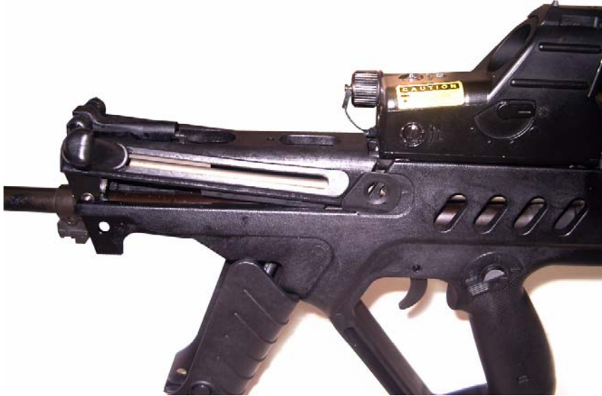
Figure 8-7. Inserting the Cocking Handle Guide Assembly
