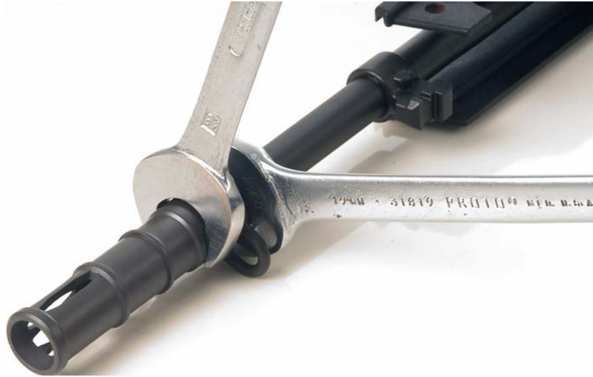
Figure 8-112. Completing the Front Swivel Sling Installation – Suppressor Tightening
