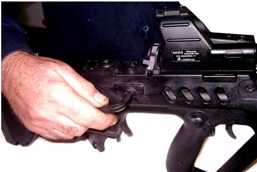
Figure 8-13. Barrel Wrench in Locking Pin
