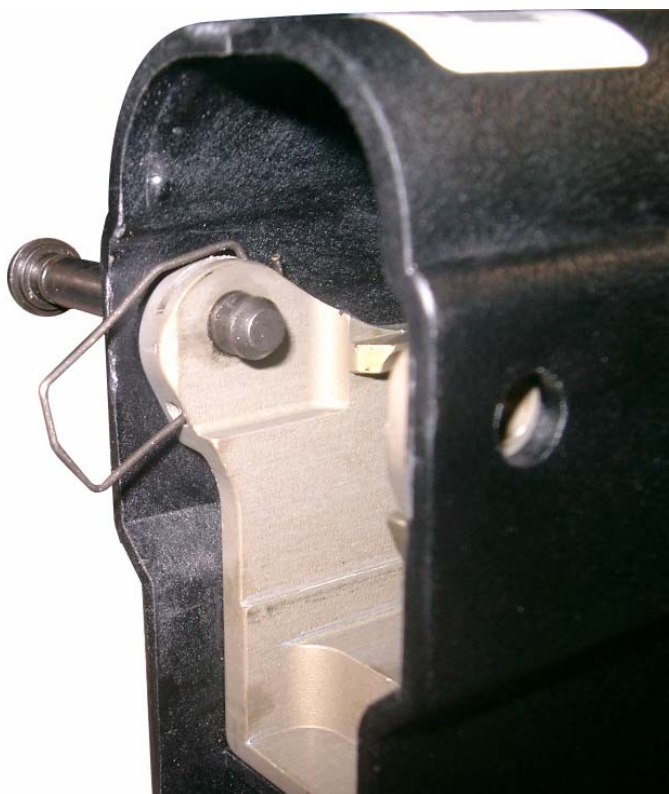
Figure 8-56. Inserting the Butt Locking Spring
