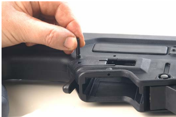
Figure 8-30. Installing the Magazine Release Lever Pivot
