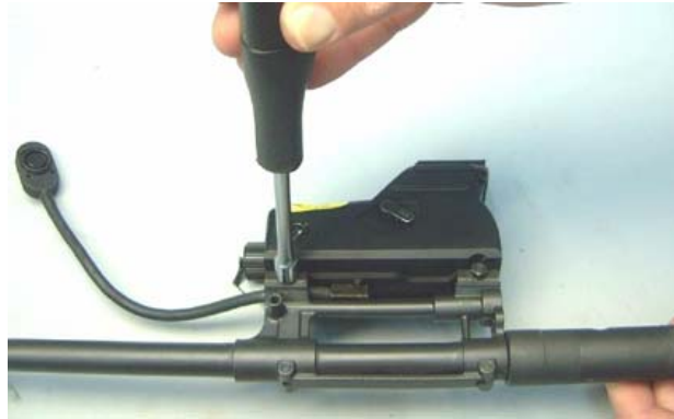
Figure 8-88. Closing the Sight Base Nuts
