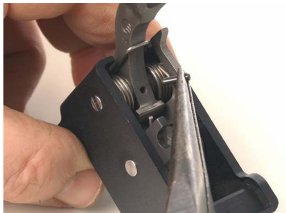
Figure 8-104. Inserting the Hammer Secure Pin
