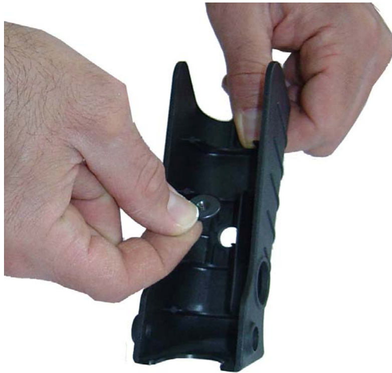
Figure 8-124. Nut and Washer Removal
