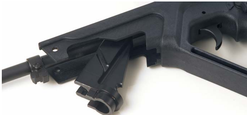
Figure 8-113. Installing the Rear Adaptor
