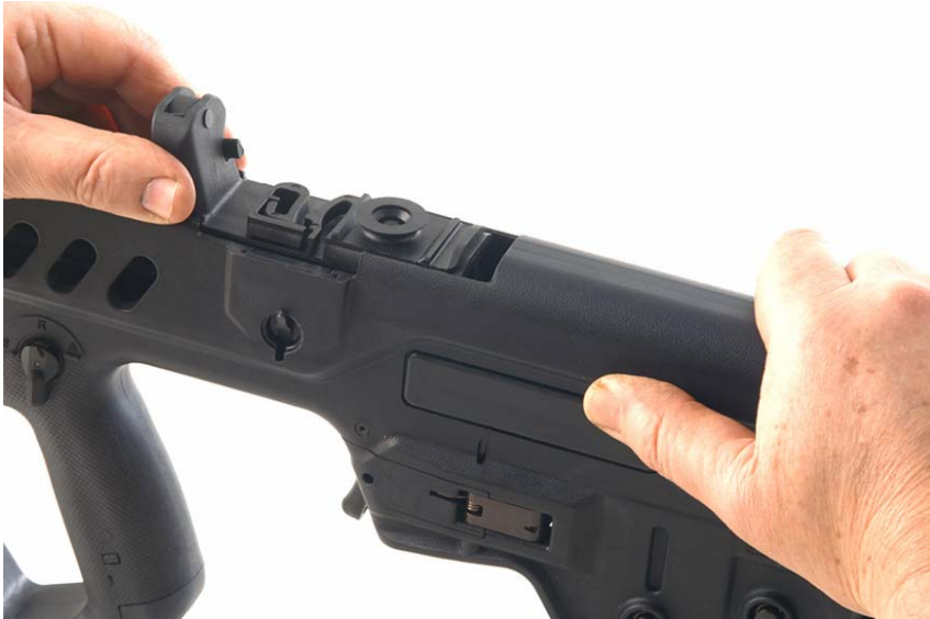
Figure 8-16. Placing Gas Cylinder into Receiver
