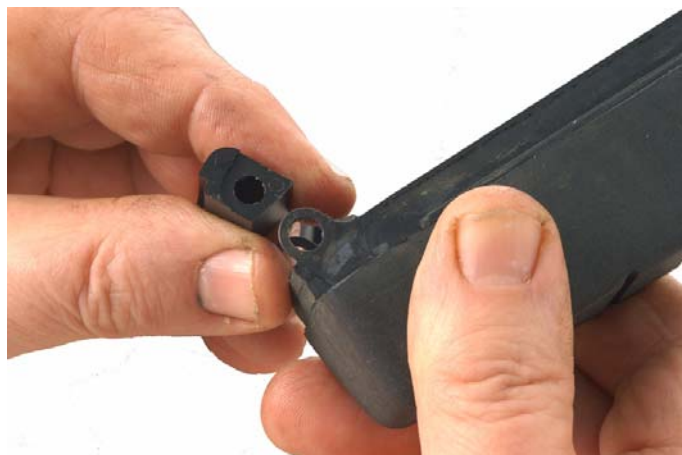
Figure 8-40. Inserting the Butt Sleeve into the Butt Assembly
