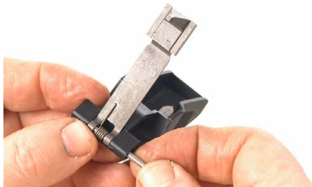
Figure 8-43. Installing Bolt Carrier Stopper Spring
