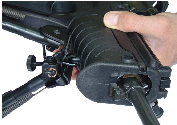
Figure 8-121. Releasing the Clamp Connector
