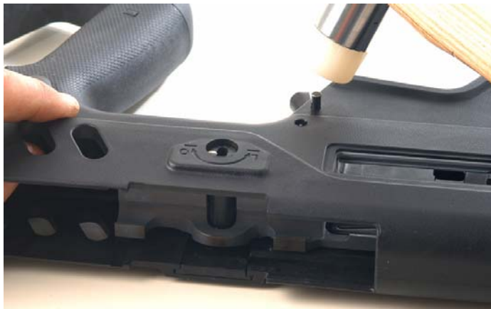
Figure 8-33. Securing the Connector Pin
