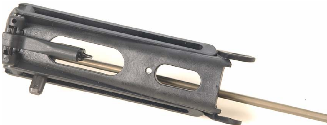
Figure 8-72. Inserting the Cocking Bar into the Cocking Handle Slot
