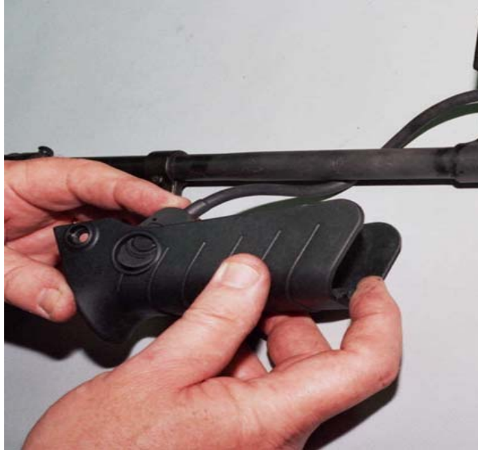
Figure 8-4. Inserting the Laser Pointer Switch
