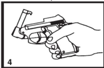
4. A tip up barrel is part of the design of this pistol. This allows the shooter to determine if a round is in the chamber or to load the chamber. Tipping up the barrel is accomplished by pushing forward on the barrel release lever.
