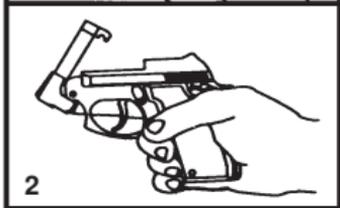
2. Tip up the barrel (by pressing forward on the barrel release lever) and check to make sure the chamber is empty.
