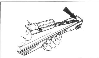
Put complete cover on frame subassembly, whereby the barrel guide must slide into the respective frame retainer. Press in protruding lock spring rod at the rear end of the cover and simultaneously press in cover until it engages into the frame subassembly.
