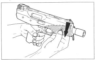
Force in lock plate to the stop and lift cover.
