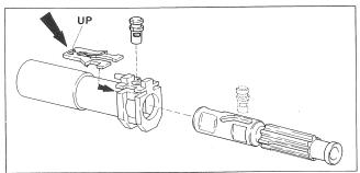
Press in lock bolt firmly with thumb and force control bolt simultaneously into the barrel guide bore to such an extent that via the control curve it locks the barrel in the barrel guide. Incorrect assembly is impossible since the control pin may be introduced in its correct position only.
