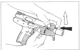
Press in lock spring rod and remove barrel, barrel guide and bolt lock. Put aside frame parts.
