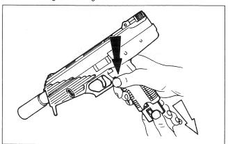
One hand is now holding the magazine. Press one cartridge with the thumb of the other hand on the magazine platform until it is retained by the magazine lips.
