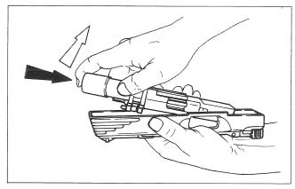
Extract barrel guide and lock bolt from cover. Remove lock spring rod and lock spring from cover. Pull cocking handle out of the cover toward the rear. Separate bolt from barrel.
