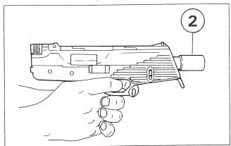
When pulling the trigger, the trigger safety is released. A shot is fired. After firing, allow trigger simply to slide forward. The gun is ready for firing again. As soon as the last shot has left the magazine, the bolt remains in its rearmost position. Remove empty magazine, slide in full magazine, release catch hold open, continue shooting.
