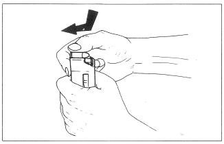
EMPTYING: Press with thumb on the bottom of the upper cartridge until it is released by the magazine lips. Now, push the cartridges one after the other out of the magazine to such an extent that they are released by the magazine lips and jump out.
