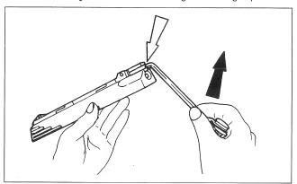
Introduce barrel/lock bolt with the end of the lock spring rod into the bore of the cover rear wall, press them against lock spring and insert them into the cover until the barrel guide engages into the cover.
