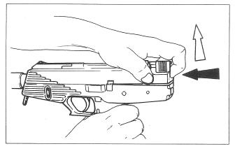
$\label{thm:cover-firmly} \mbox{Hold cover firmly in one hand. Press barrel guide, while lifting it, against bolt spring.}$
