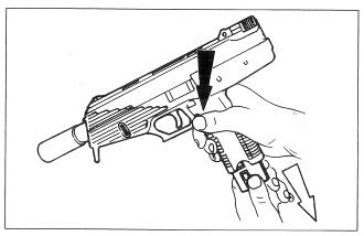
Pull cocking handle firmly backward so that the cartridge being in the barrel is extracted and ejected. Simultaneously press catch hold open upward so that the bolt is locked.
