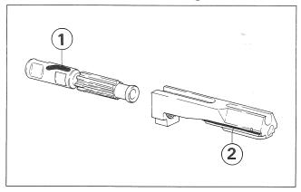
Wipe off the plastic parts with a dry cloth only. Before shooting, the barrel has to be de-oiled.
