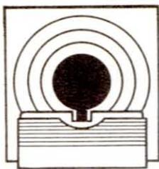
5. LINE the sights carefully, top of front sight even with top of rear notch, and light equal on both sides of front sight (see illustration).
