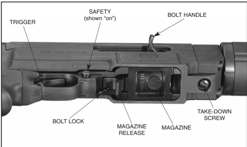
**Figure 2.** In these illustrations the frequently used operating components are identified. Note that the safety is protruding fully from the right side of the trigger guard and is therefore in its "on" (safe) position.
