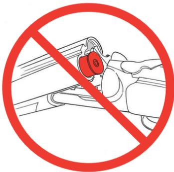
So that the gun can be conveniently reloaded after firing one shot, the selective ejector mechanism only ejects fired shells. It does not eject live ammunition. Do not rely upon the ejector mechanism to unload the gun. Simply opening the gun does not unload it. To unload, open gun smartly, manually remove all cartridges, and visually check both chambers to be sure both chambers are unloaded.
