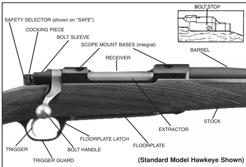
**Figure 1.** Right-handed version shown. In this illustration the cocking piece is shown cocked (protruding from the rear of the bolt sleeve). The bolt stop (on the left side of the receiver) permits the bolt to be withdrawn simply by pulling it out to the left. **The safety selector should be in the “Load-Unload” position when the bolt is being removed or installed.**
