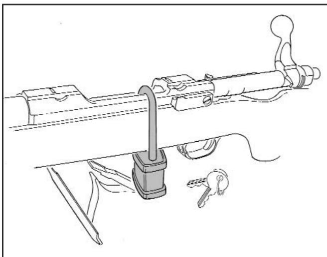
***Correct Installation of Lock
