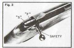
TO LOAD MAGAZINE — Put safety ON SAFE. Remove clip magazine by pushing rearward on magazine latch (Fig. 4) and pulling clip from bottom of rifle. Load cartridges into magazine. When fully loaded, magazine will hold five (5) cartridges. To replace magazine, fit channel opening on back of magazine over end of magazine guide. Push magazine upward until locked into place by magazine latch.
