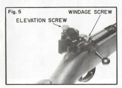
WINDAGE — Turn the windage screw (Fig. 5) clockwise to move eyepiece left or counter clockwise to move right. NOTE: Always move the eyepiece in the same direction as you need to move the bullet on the target.
