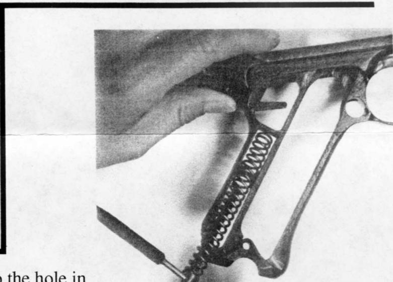
**21.** Insert a drift of the proper size into the hole in the lower end of the recoil spring guide, working from the right side of the frame. Push the recoil spring up (toward the top of the frame) to free the lever from the hook on the spring guide, then ease the spring and guide out toward the right for removal. **Caution:** The recoil spring is under some compression, even at rest, so take care that it doesn't get away.
