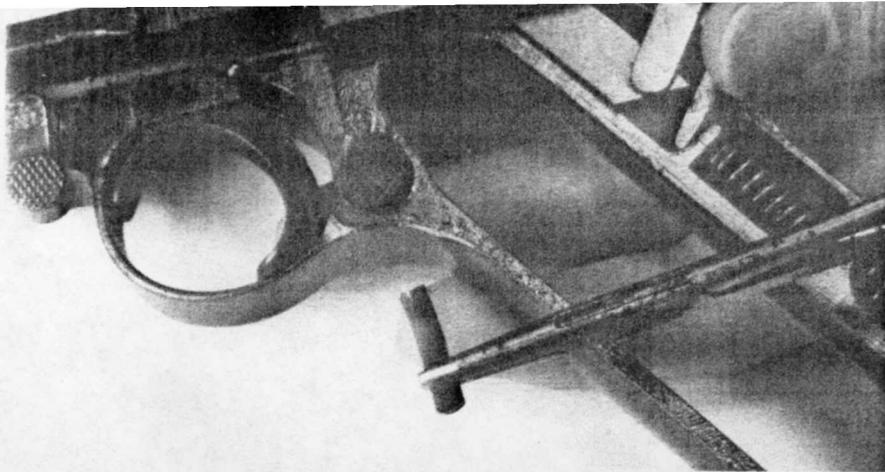
15. Use a small screwdriver to slightly depress the upper end of the magazine catch spring, and push the spring forward from beneath its shelf in the frame. Removal of the spring will free the magazine catch.
