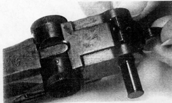
Slide the breech block and toggle assembly out of the rear of the barrel extension. The gun is now field stripped.
