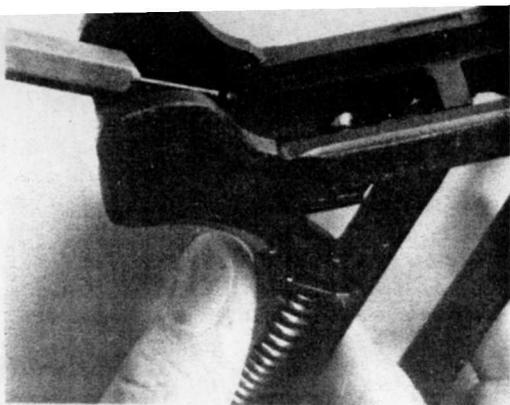
**20.** Driving out the small pin located inside the left rear of the frame
