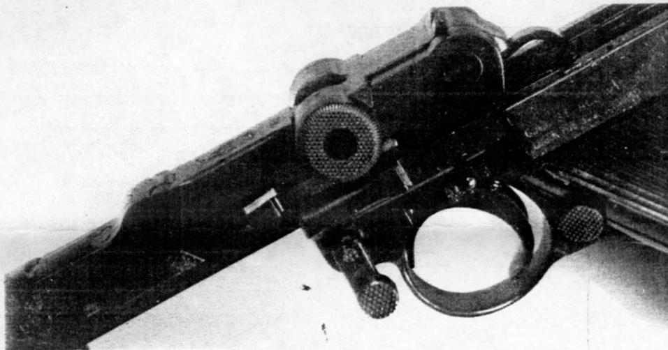
**3.** Remove the barrel and bolt assembly forward off the frame.
