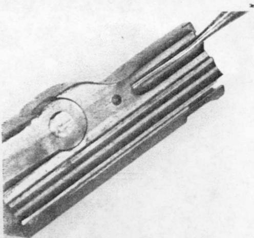
**8.** Drifting out the small cross pin in the breech block will release the extractor and its spring for removal.
