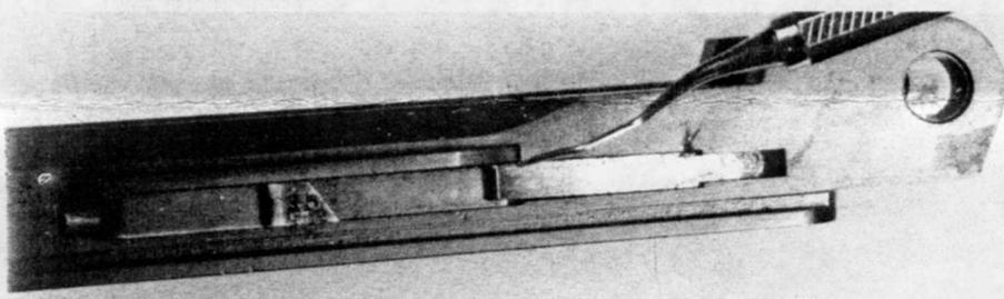
**10.** With a small screwdriver, lift the hooked end of the sear spring just enough to clear the step on the sear tail, and slide the spring forward to remove it.
