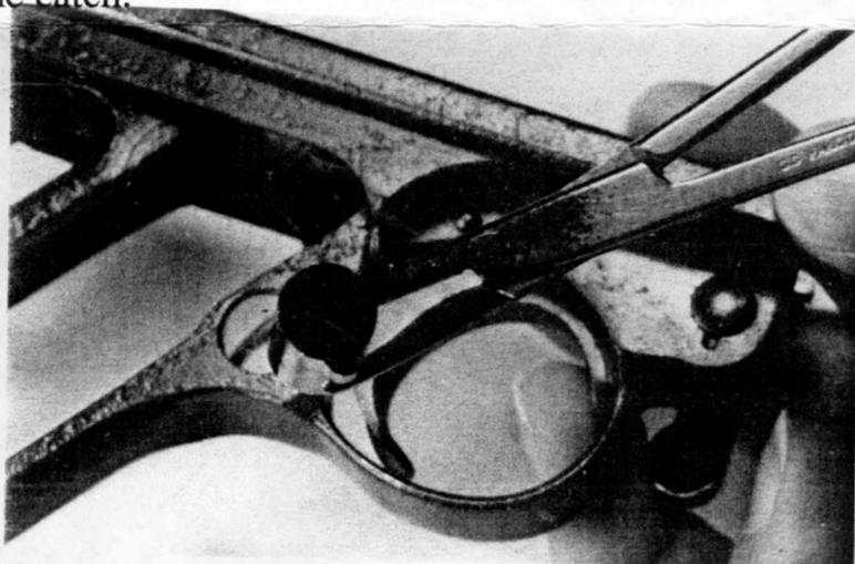
17. The takedown lever can be pushed from the right side of the frame and removed toward the left. The tip of its retaining and positioning spring can be drifted inward from the front underside of the frame for removal.
