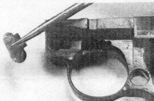
18. The trigger may easily be moved to the left and taken out of the frame, along with its attached spring.
