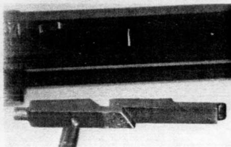
**11.** Remove the sear assembly from the left side of the barrel extension.
