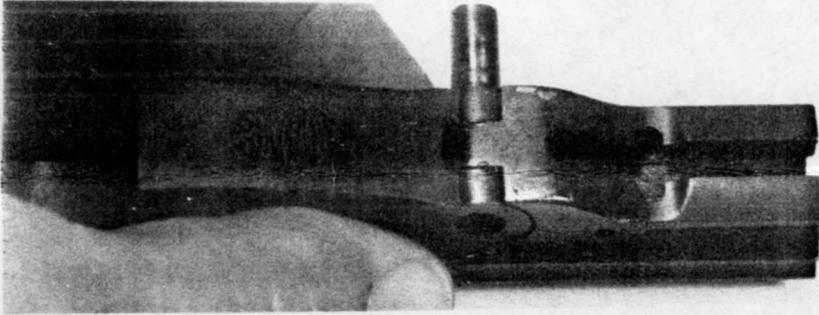
**6.** Remove the front cross pin of the toggle assembly to free the breech block for removal. **Note:** In some cases, this pin will be very tight. Do not force it as this could cause deformation or breakage of parts.
