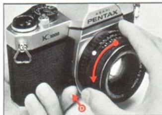
**4.** To detach, hold the camera with your left hand. Depress the lens release lever **D** while turning the lens counter-clockwise with your right hand.
