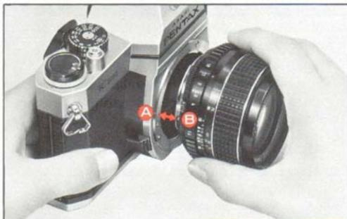
1. To remove the Mount Adaptor K from the camera body, first remove the screw-mount lens. Then press, with your thumbnail or a pointed object such as a ballpoint pen, against the spring pin **C**.
