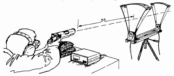
The first skyscreen the bullet will pass over should be plugged into START, the second screen should be plugged into STOP.
