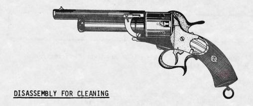
CAVALRY MODEL - Lower the lever latch located at bottom front of frame. The barrel will then fully unscrew in a counter - clockwise direction.
