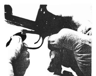
26. The cylinder-stop spring is dovetail-mounted in the front of the guard. If necessary for repair, it can be drifted out toward the rear.
