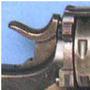
In 1883, a new cheaper Nagant model was used by the Belgian Army. The cylinder periphery was plain, without the usual lengthwise flutes, and the lock was of single-action type as shown in the two pictures here (the hammer must be thumb-cocked for each shot). Also, the hammer was of rebounding type. In the picture on the left, the hammer is positioned slightly rearward when the trigger is released.
