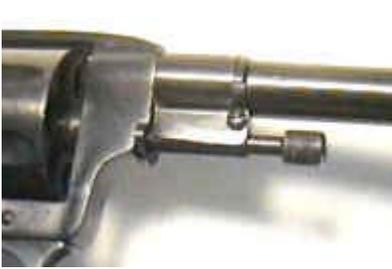
ejector rod under the barrel
