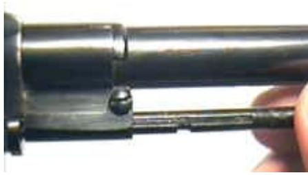
bolt notch on the ejector rod
