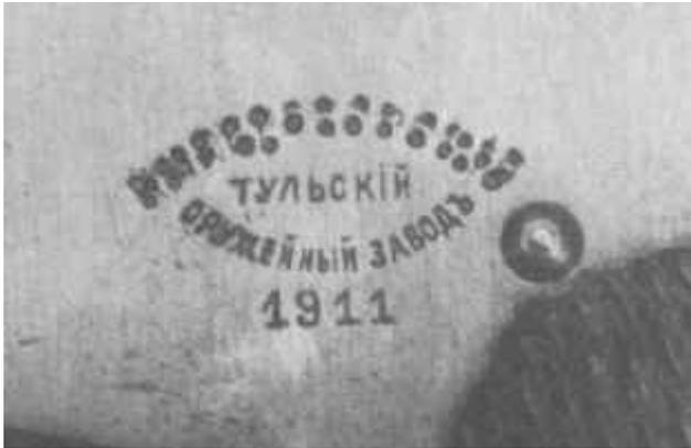
First line of the marking, punched out
