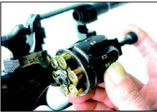
In the Nagant case, every spent cartridge had to be pushed out individually by the ejector rod that pivoted around the barrel. Moreover the rod was even not equipped with a return spring. This obsolete feature for a service revolver made the loading and unloading operation both lengthy and very tedious. Many Russian officers were very happy to keep their old easy-to-load and powerful Smith & Wesson revolvers when fighting against Japan (1904-1905) and even as late as WW I against Germany.
