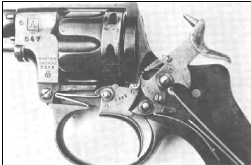
The model 1878 shown here was chambered for the 9.4 Nagant cartridge. The lock mechanism was of double-action (trigger cocking). As most revolvers of the same period it included a lot of parts and springs. The sear for example was a separate part with its own return spring (colored in red on the patent drawing above).
