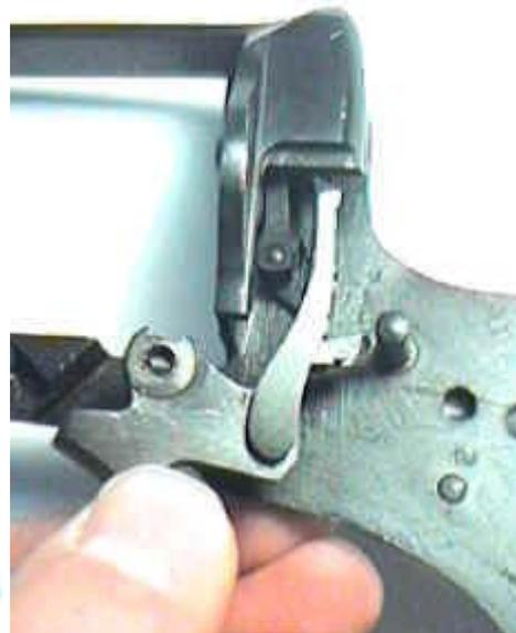
cylinder hand clearing the frame shield
