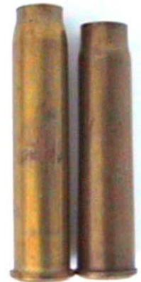
The Pieper 7.62 mm ammunition is 41 mm long (Nagant : 38.8 mm).
