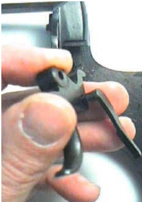
removing of the cylinder hand from the trigger
