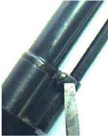
ejector rod spring retaining screw - after takedown
