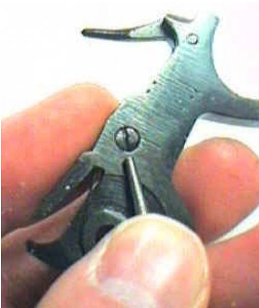
double-action hammer with a strut
