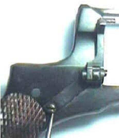
loading gate spring retaining screw
