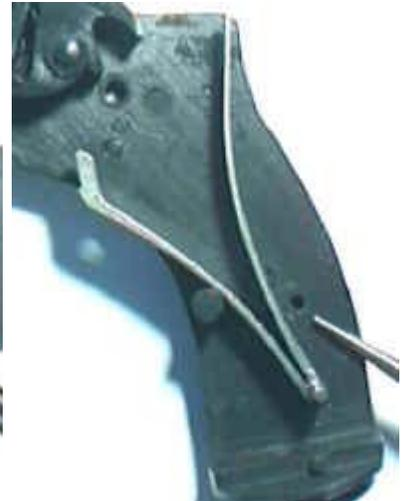
**Tip the hammer back to clear the frame and lift it off. The mobile firing pin is retained on the hammer with a cross-pin, but removing it is not advisable in normal takedown. Tip the cylinder hand back to clear the frame and lift the trigger off. The cylinder hand is easily detached from the trigger**
