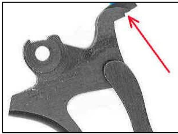
The picture below shows the position of the parts after the hammer was thumb-cocked, and caught by the sear (red arrow here-left), which is an integral part of the rear arm of the trigger.
