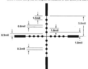
horizontal reticle over the target instead of the crosshairs. By choosing the correct dot, you can easily adjust for how much the point of impact will drift in the wind.
