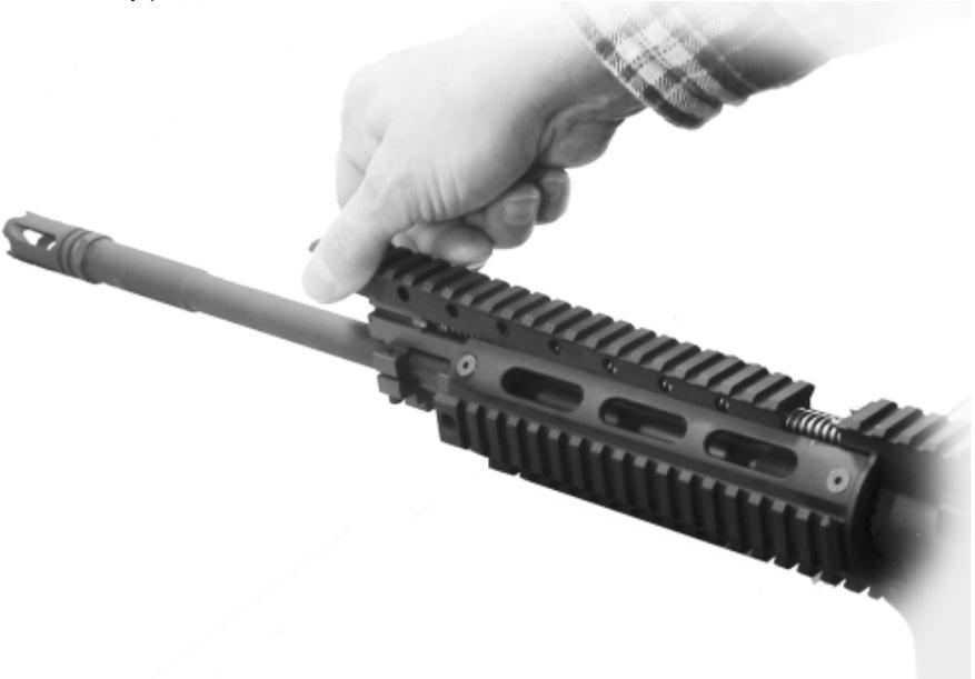
5. Retract the spring to release it off the spring clip, as shown. Push the spring clip back towards the spring and lift it upwards to remove it from the op-rod. It may necessary to gently tap the spring clip to release it.
