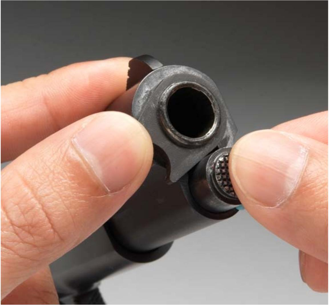
**Figure 5. Remove the Recoil Spring Plug**
