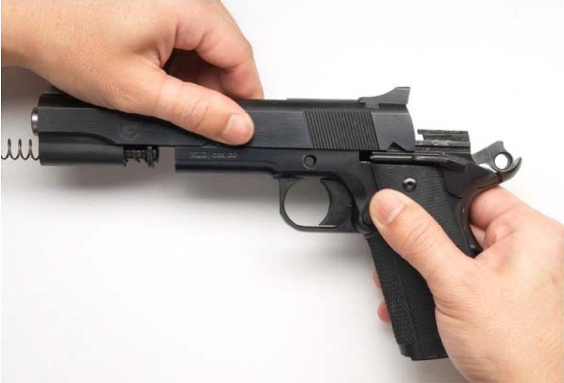
**Fig. 7 Remove the Slide**
