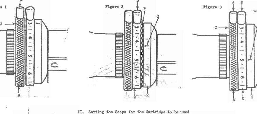
Figure 1 - Loosen the slotted head knob (A) and slotted head screw(B) and pull range ring (C) to the
