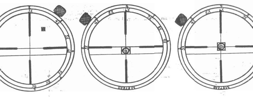
NOTE: A target 18" (inches) in height must be used to "Range" the scope
