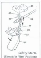
If your Kimber is a Series II firearm, then it is supplied with an integral firing pin block. This feature does not allow the firing pin to be active until the Grip Safety is depressed. THIS ADDED SAFETY DOES NOT ELIMINATE THE NEED FOR SAFE AND PROPER GUN HANDLING. READ THIS OWNERS MANUAL THOROUGHLY.
