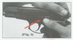
the slide release lever in it's notch in the slide (Fig. 3).
