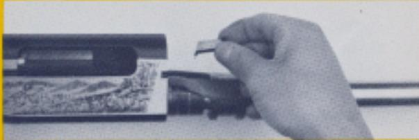
7. A sharp pull straight out on the charging handle will release it from the bolt. Slide the gas sleeve and the action bar forward off the magazine tube. **NOTE:** Carbon buildup on the magazine tube may make removal of the gas sleeve difficult. If so, use 00 steel wool soaked in cleaning solvent to remove excess carbon from the magazine tube. Wipe dry with a clean cloth.
