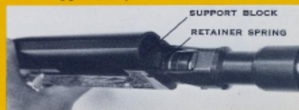
6. At the forward end of the receiver is the support block and the support block retainer spring. Rotate this spring
