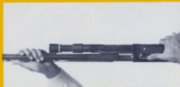
3. With the bolt still in the open position slide the barrel ring over the magazine tube and barrel into the receiver. Be sure the barrel is fully seated in the receiver.
