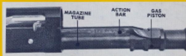
9. Clean all parts by washing with a good solvent and wipe dry with a soft cloth. Oil all friction points on trigger and bolt assemblies with a good light oil. **Do not** oil magazine tube or gas sleeve. Barrel may be cleaned with a proper
