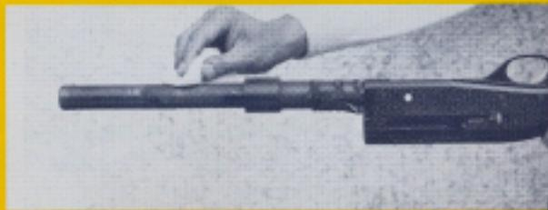
8. The action bar may be removed from the gas sleeve by lifting the rear to disengage the locking cams.
