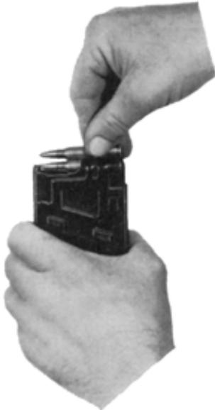
Fig. 28 Filling of magazine
