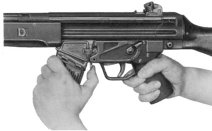
Fig. 32 Removing of magazine
