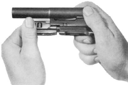
Fig 41 Disassembly of bolt
