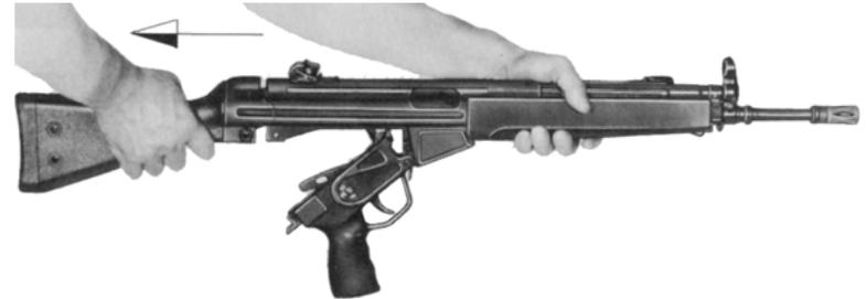
Fig. 39 Removal of butt stock
