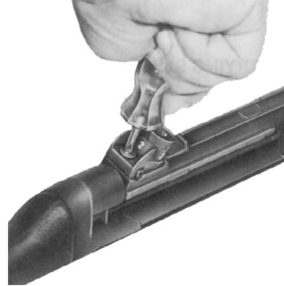
Fig. 45 Loosening of clamping screw
