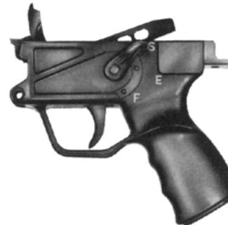
Fig 15 Grip assembly and trigger mechanism
