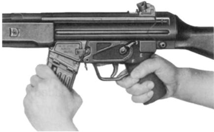
Fig. 31 Inserting of magazine
