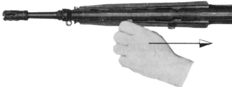
Fig. 33 Retracting of cocking lever
