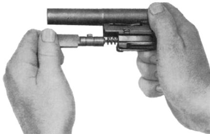
Fig. 42 Extracting the locking piece, firing pin and firing spring
