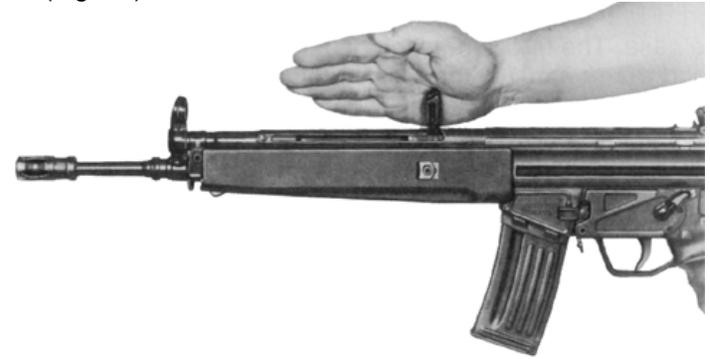
Fig. 34 Cocking lever snapping forward
