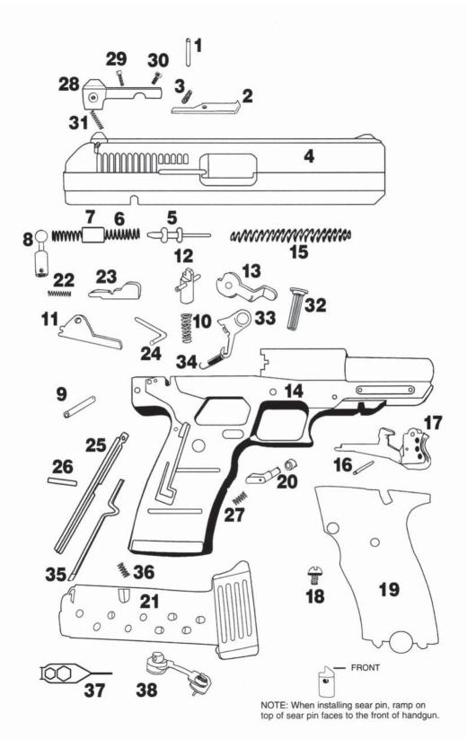
Safety/Slide Lock is located at top of left grip. Sliding safety lever upward, into notch engages safety, exposes letter (S) on grip and places pistol in "SAFE" position.
