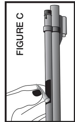
slide down toward the action. Do not exceed the capacity of the magazine. Next, push the inner magazine tube back down into position and lock into place. Please be careful when pushing the inner magazine tube in, as it is under spring tension.
