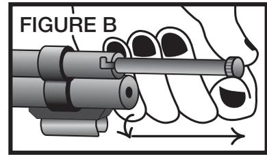
B) and pulling the tube out until the orange follower (black on magnums) is visible through and clears the loading port in the outer magazine tube. With the muzzle pointed upward, insert the rimmed end of the cartridges into the magazine (Figure C) and allow them to slide down toward the
