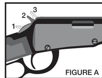
The hammer will now be locked into the Safety position and, if you pull the trigger to fire, the hammer should not fall. The essential maneuver of setting the Safety this way is to remove your finger very quickly from the trigger
