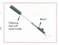
Be careful not to scratch or damage the muzzle as this can affect accuracy: it is recommended to clean from the rear side.
