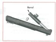
This level of disassembly is sufficient to perform thorough cleaning: further disassembly should only be carried out by an authorized armorer or by FN HERSTAL
