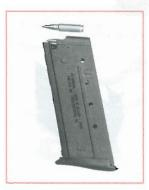
Place the cartridge on top of the lips of the magazine and with its rear part aligned with the rear of the magazine
