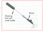
Be careful not to scratch or damage the muzzle as this can affect accuracy . It is recommended to clean from the rear side.
