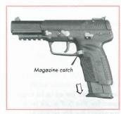
The magazine pops out when pressing the magazine catch, standardly provided on the left side of the pistol.
