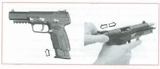
Being extremely careful not to touch the trigger, hold the pistol in your firing hand, point in a safe direction, pull the slide completely rearwards with the other hand and then release the slide which returns under spring force.
