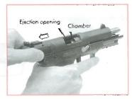
Through the ejection opening, look into the chamber of the pistol in order to ensure that there is no cartridge in the chamber.
