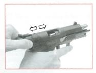
If the slide is already automatically locked into the rearward position after having fired the last round (also refer to § 4.7), this step is not necessary: just press the slide release lever dawnwards in order to let the slide return to its forward position.
