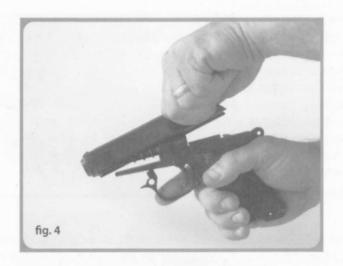
The slide assembly may then be drawn forward and removed from the barrel (fig. 4). The recoils spring may be removed by pulling it off the front of the barrel. No further disassembly is required or recommended for cleaning purposes. Further dismantling is a job for qualified gunsmiths and armourers only.
