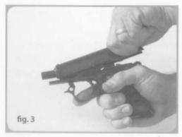
Holding the pistol with the right hand, grasp the grooved surfaces at the rear of the slide with the left hand and pull the slide fully to the rear. Lift the rear end of the slide assembly out of the receiver rails (fig. 3).
