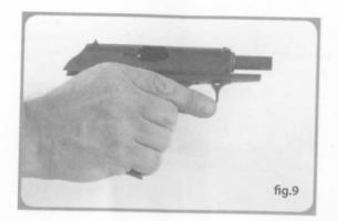
**6. Reloading** during shooting: when the magazine is empty, the slide is held open (fig. 9).
