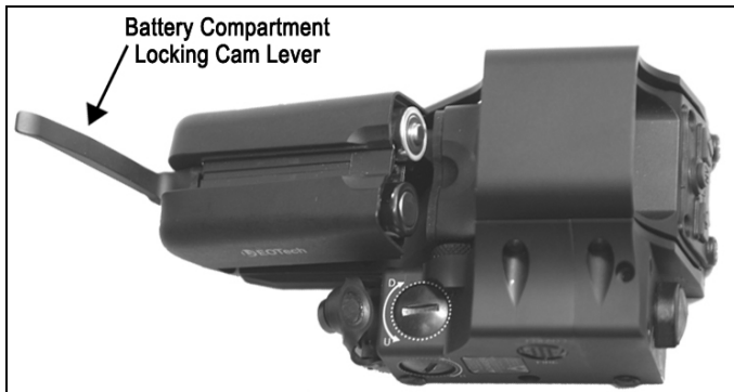
Figure 3-1 EOLAD Battery Installation
