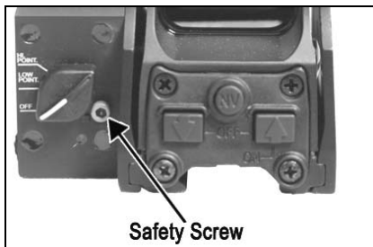
Figure 3-3 Laser Safety Screw Installed
