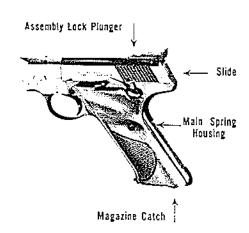
MAGAZINE. The magazine has an easily operated thumb-piece which greatly facilitates loading. The magazine is held in the receiver by a magazine catch at the base of the main spring housing. Thumb pressure on this eatch releases the magazine.
