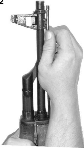
5. Remove the receiver cover. Lean the rifle against a table and hold the forward part of the butt with the right hand, depress the guide face with the thumb into the cover hold and raise the cover with the left hand (Fig 3).
