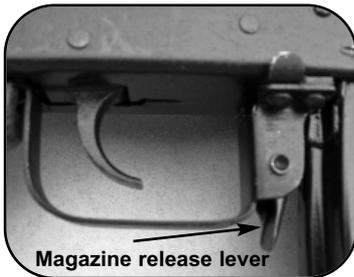
Press the magazine release lever forward to remove the magazine from the rifle.
