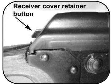
The receiver cover retainer button is used to start the disassembly process.
