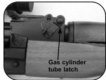
Rotate the gas cylinder tube locking latch upward to free the gas cylinder tube.
