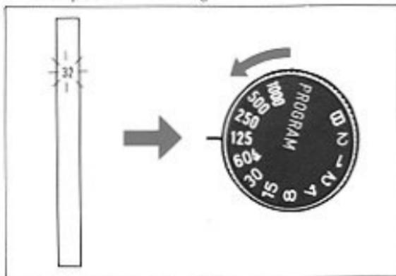
**Shutter-speed priority AE mode:** "32" blinks regardless of the minimum aperture of the lens in use. Choose a faster shutter speed until the display stops blinking. When using a lens whose minimum aperture is  $f/22$  or  $f/16$ , even when "32" does not blink, turn the shutter speed selector dial until a number equal to or smaller than the lens' minimum aperture is displayed.
