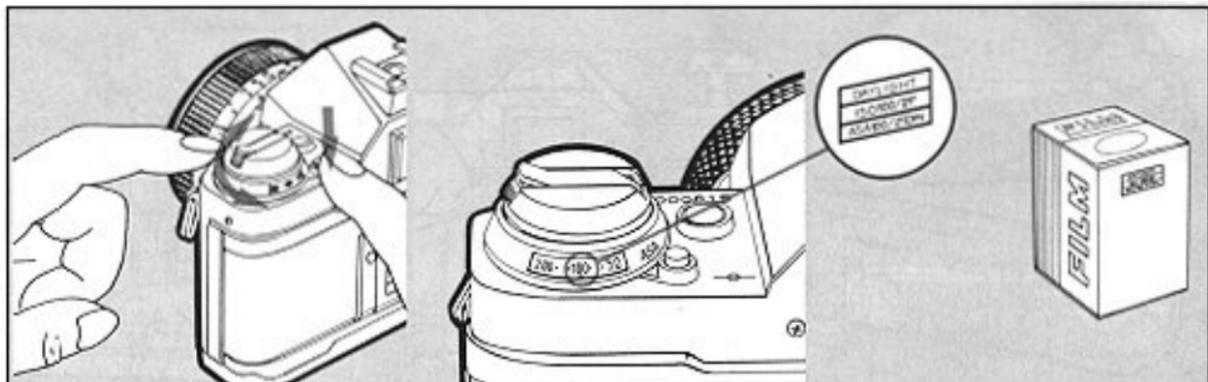
While pressing the lock release button, slide the ASA setting lever until the ASA speed of your film is aligned with the green index. This is necessary for getting correct exposure.
