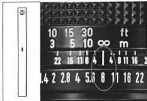
You can roughly check the depth of field visually with an FD lens as follows:
