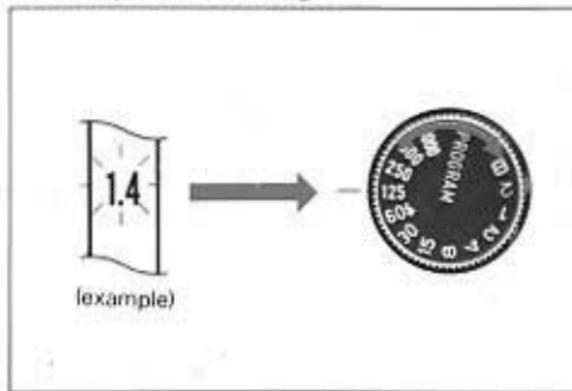
**Shutter-speed priority AE mode:** A number equal to or smaller than the lens' maximum aperture blinks. Choose a slower shutter speed so that the aperture stops blinking.
