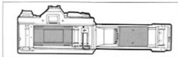
While loading the film, take care not to touch the shutter curtain, the film rails or the pressure plate (shown in red).
