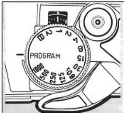
Turn the shutter speed selector dial until "PROGRAM" is aligned with the index.
