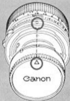
Turn the rear lens cap in the direction of the arrow until it stops and pull it off the lens.
