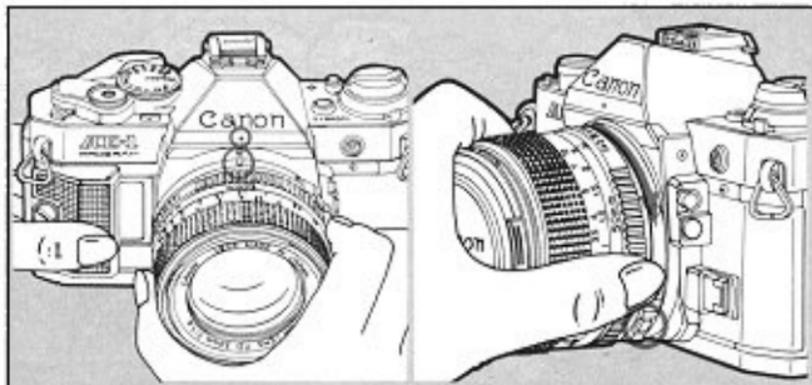
To mount the lens, first align the red positioning point on the lens with the red dot above the camera mount as illustrated.
