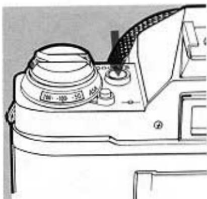
If you have started the self-timer and wish to cancel it before shutter release, press the battery check button or push the main switch back to "L."
