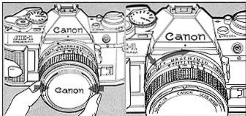
Remove the front lens cap.
