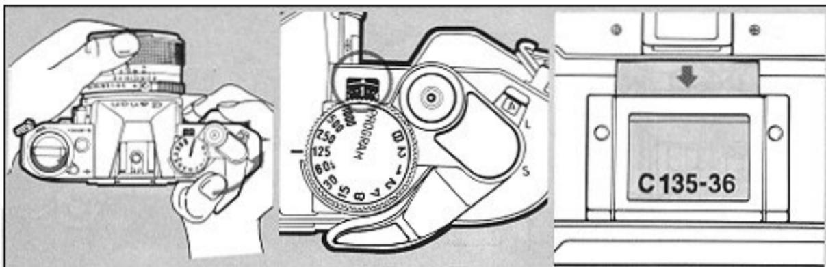
Take several blank shots, releasing the shutter and advancing the film, until the frame counter reads "1." While doing this, keep an eye on the rewind knob. If it rotates in the direction of the arrow, the film is loaded correctly.
