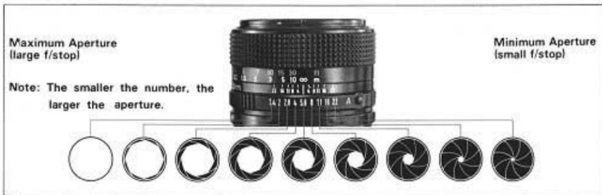
[Example Shown: FD 50mm f/1.4. Maximum and minimum apertures differ depending on lens]
