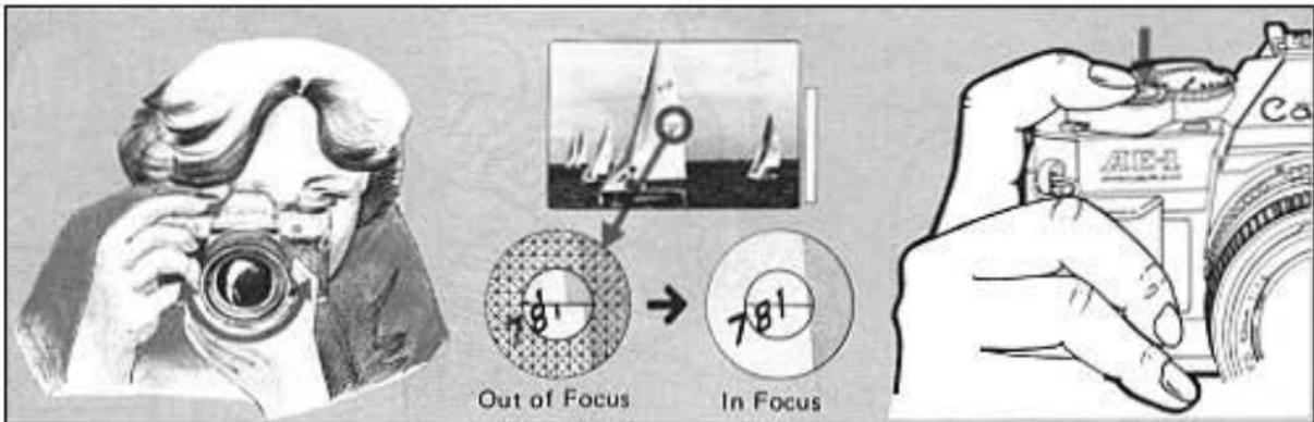
Turn the focusing ring until the main subject is sharp and compose the picture.
