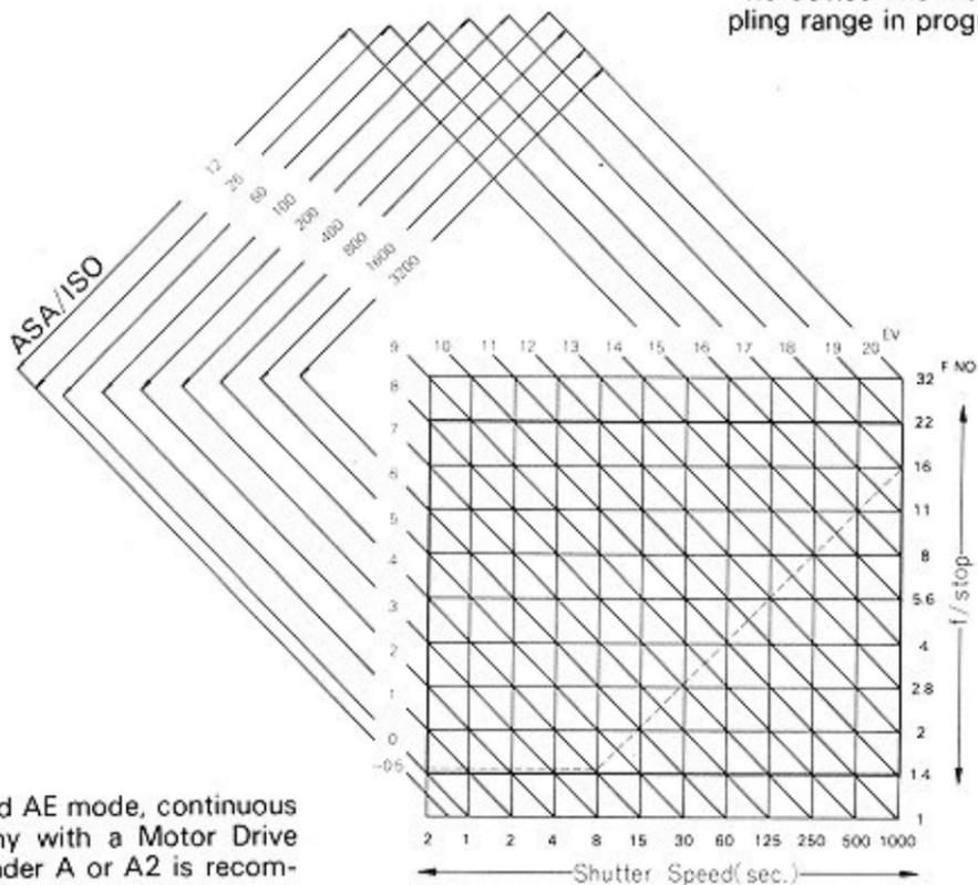
In the programmed AE mode, continuous frame photography with a Motor Drive MA or Power Winder A or A2 is recommended only if the light is bright enough to give an aperture display of f/4 or larger. In this case, the shutter speed will be at least 1/60 sec.
