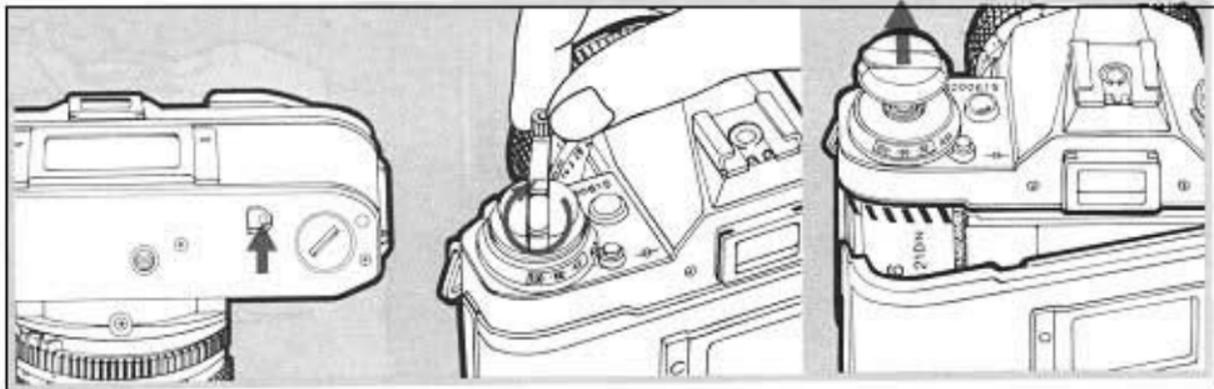
You can tell you have reached the end of the film by the frame counter and the film advance lever. Either the film advance lever will not turn at all or it will not turn all the way. First press in the rewind button.
