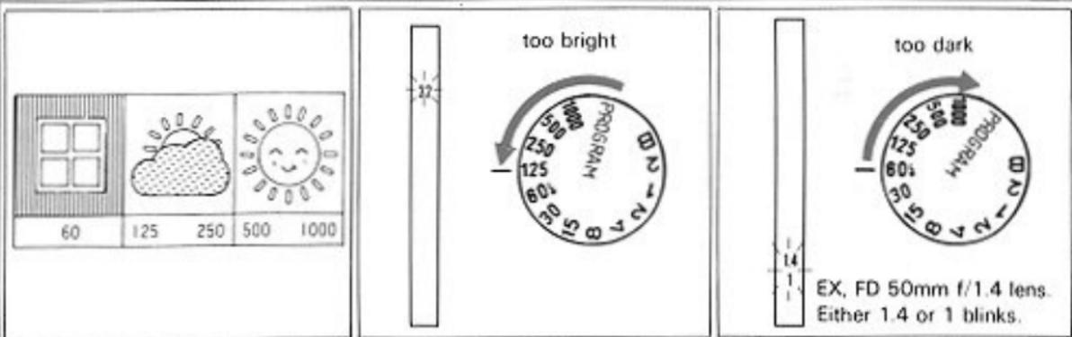
Turn the shutter speed selector dial from "PROGRAM" and set a shutter speed. Refer to the illustrations above when choosing a shutter speed. While looking in the viewfinder, press the shutter release button halfway. Exposure will be correct as long as the aperture display does not blink.
