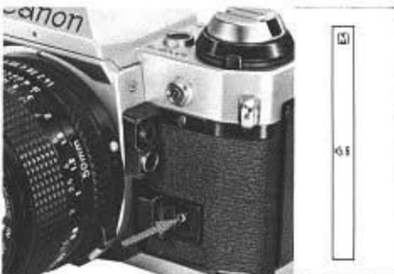
With a Canon FD lens, metering is done with the lens diaphragm at its widest opening. This is called "full-aperture metering."
