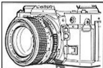
To remove the lens, turn it in the direction of the arrow, while pressing the lens release button, until it stops.
