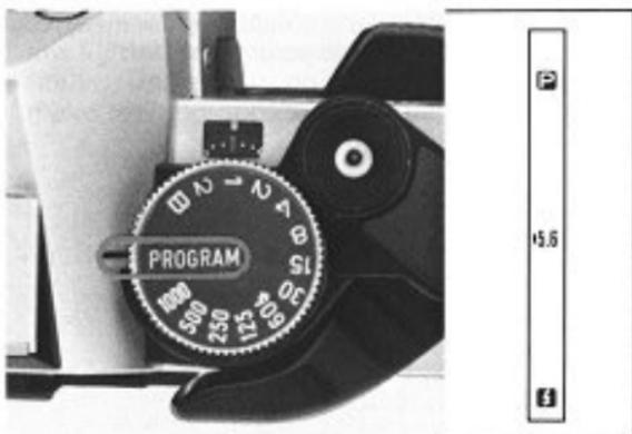
When the lens' aperture ring is set to "A" and the shutter speed selector dial to "PROGRAM," a green "P" LED 5 is displayed, indicating programmed AE photography. If the shutter speed selected automatically by the camera is 1/30 sec. or slower, the "P" will blink. This is to warn you that your picture may be blurred due to camera movement if you are hand-holding the camera.
