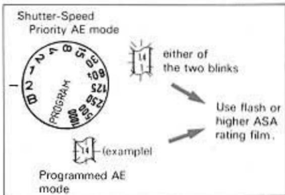
**Shutter-speed priority AE mode:** When 2 sec. is set on the shutter speed selector dial and a number equal to or smaller than the lens' maximum aperture blinks; or
