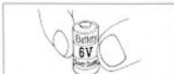
Do not touch the battery terminals. Wipe them and the camera contacts with a clean, dry cloth before loading to prevent poor contact from dirt.
