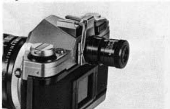
The Magnifier S gives a 2.5X magnification of the center of the viewing area for precision focusing in close-up work and wide-angle photography. Its power is adjustable to your eyesight within a range of +4 to -4 diopters. Its adapter is hinged so that the magnifier can be swung upward from the eyepiece, leaving the entire screen image visible.
