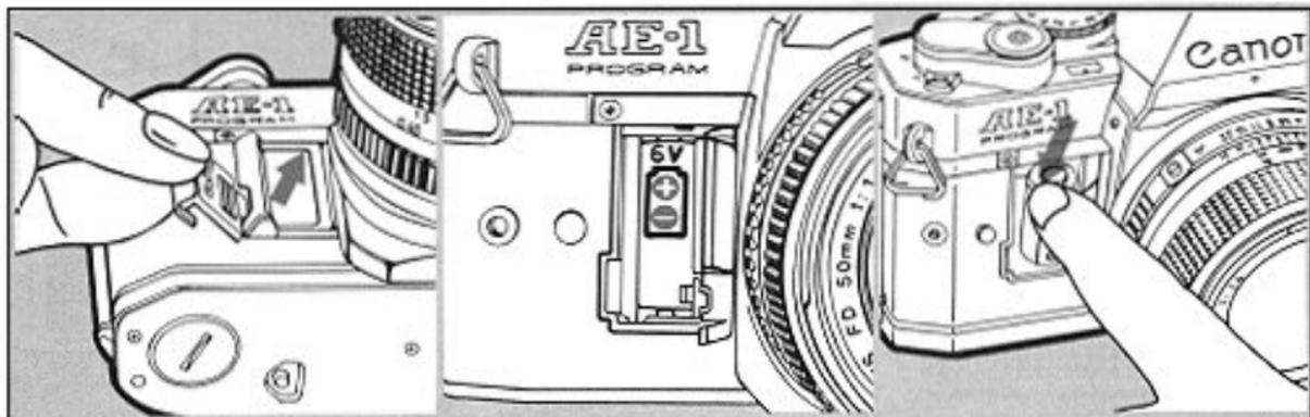
Open the battery chamber cover using the viewfinder cover.
