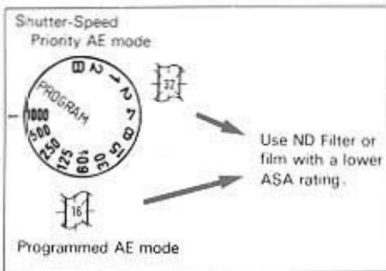
**Shutter-speed priority AE mode:** When "32" blinks and the shutter speed selector dial is set to 1000; or
