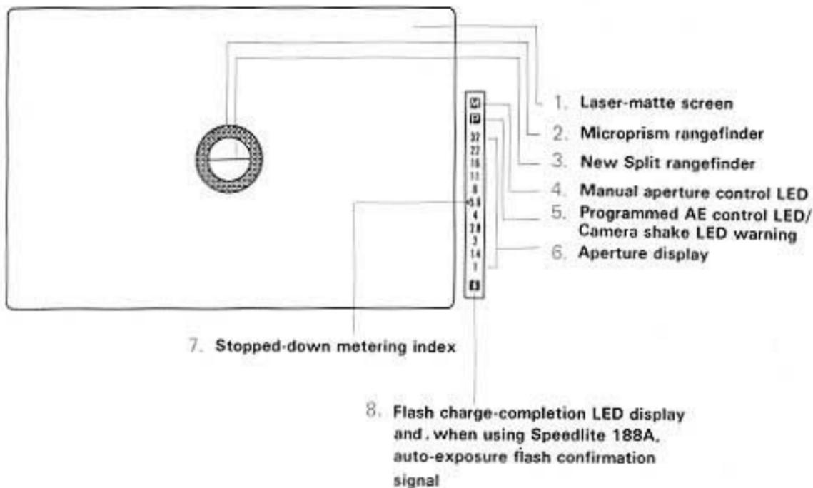
The AE-1 PROGRAM's viewfinder is especially bright to facilitate viewing and focusing. It displays only the necessary information, using a Light-Emitting Diode (LED) system of illumination. The degree of LED illumination changes in four stages depending on the brightness of the subject. When the subject is brighter, the LED brightness is slightly higher; it is slightly lower with a darker subject. Thus the LED maintains an almost consistent degree of brightness to the human eye.
