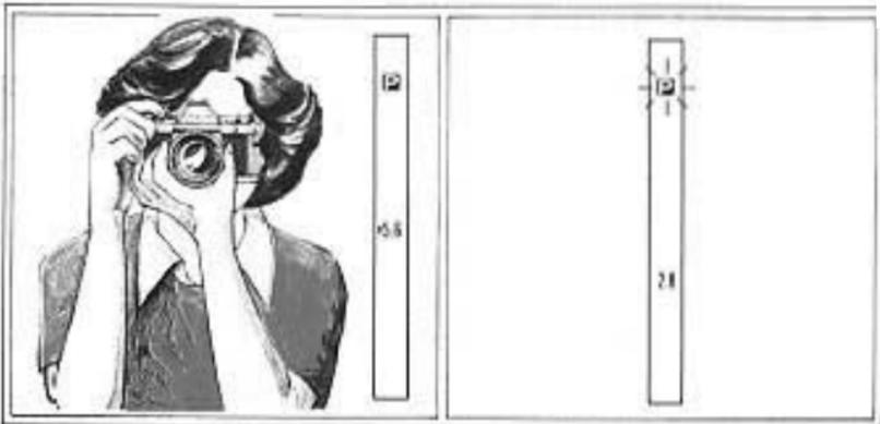
Look into the viewfinder and press the shutter button half-way. A green "P" and a number will appear to the right of the field of view, indicating programmed AE and the aperture selected automatically by the camera.
