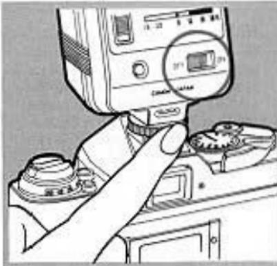
Make sure the main switch on the flash is OFF. Then slide the flash into the AE-1 PRO-GRAM's accessory shoe. Tighten the lock nut.
