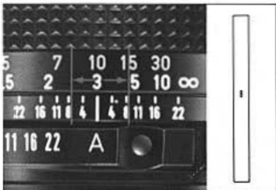
There are two ways to check the depth of field. The usual one is by using the depth-of-field scale on the lens. This is a scale of f/stops repeated on each side of the distance index.
