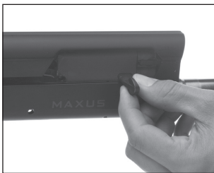
Pull outward to remove the bolt handle.
