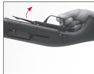
Lift the trigger group from the receiver.
