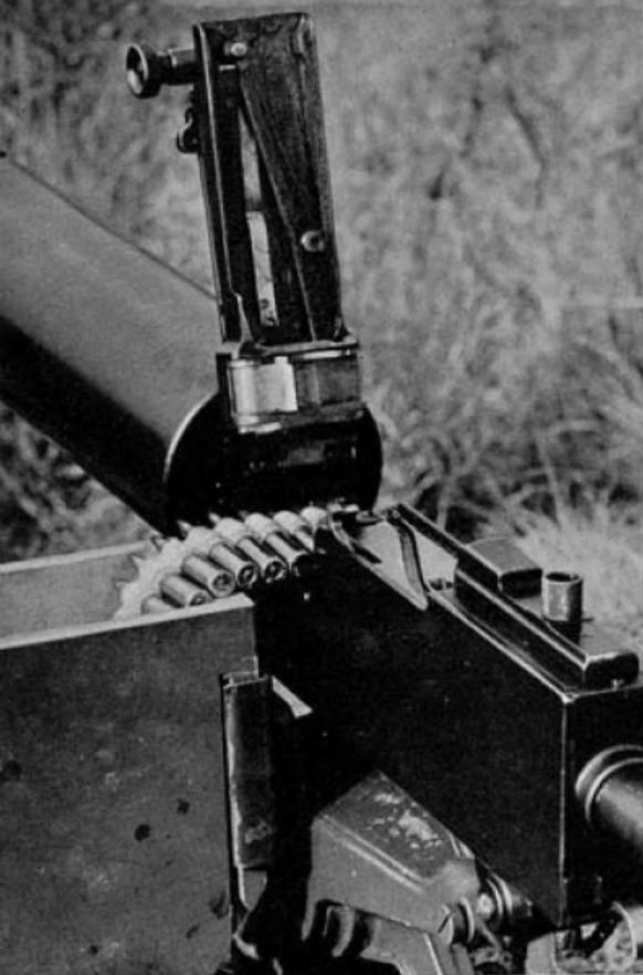
**TOP ILLUSTRATION :** Shows bolt in fully forward position. Cover raised to show the belt feed arm actuating stud, having been driven to the left when located in cam groove of bolt. Thus the forward end of the belt feed arm has driven belt feed pawl to right, thus positioning succeeding round against cartridge stops in feed way. The extractor is gripping succeeding round.
