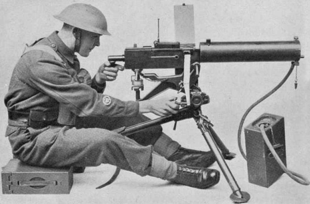
PLATE 13 *The Firing Position (Gun mounted on 1918 Tripod)*
