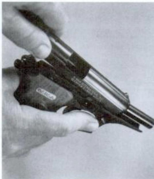
2. Draw the slide back all the way and lift it up at the rear. The slide can then be moved forward off the barrel and frame, and the recoil spring can be removed from the barrel. Gun is now field-stripped.
