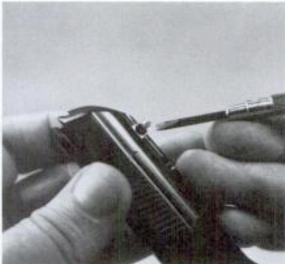
5. With a non-marring tool, the rear sight can be drifted out of its dovetail toward the right. The sight leaf can be taken out of the base by backing out the adjustment screw. Take care that the small coil spring behind the bottom of the leaf isn't lost.
