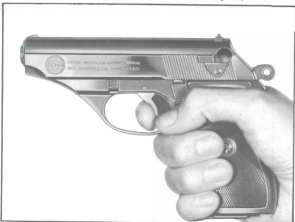
After the first shot has been fired the pistol functions semi-automatically, utilizing the recoil from each shot to push the slide rearward, extract the fired cartridge case from the chamber and eject it from the pistol through the ejection port. The rearward movement of the slide also cocks the hammer. The forward re-
