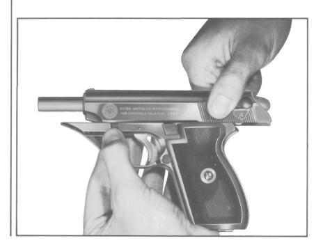
Lift up the rear of the slide and allow it to move forward to clear the front of the barrel. The recoil spring may now be removed. Never allow the hammer to drop forward onto the frame while in this dismantled condition as damage to the pistol may result. Further disassembly is not
