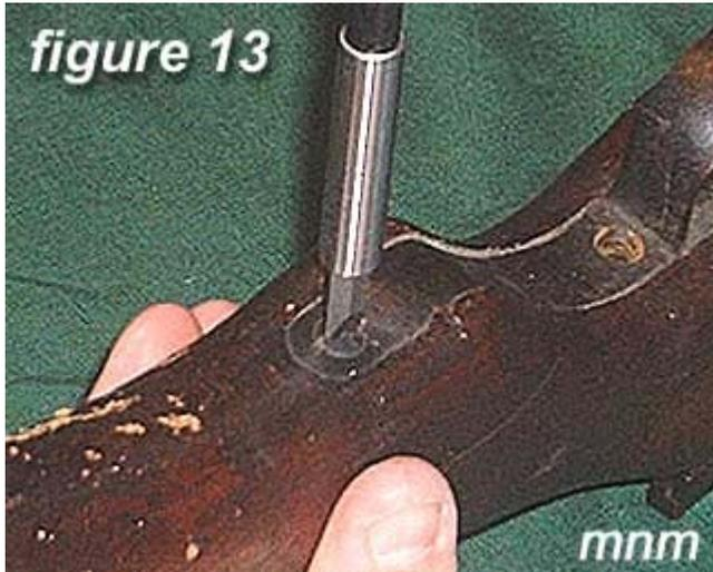
13) Remove the **rear trigger guard screw**.
