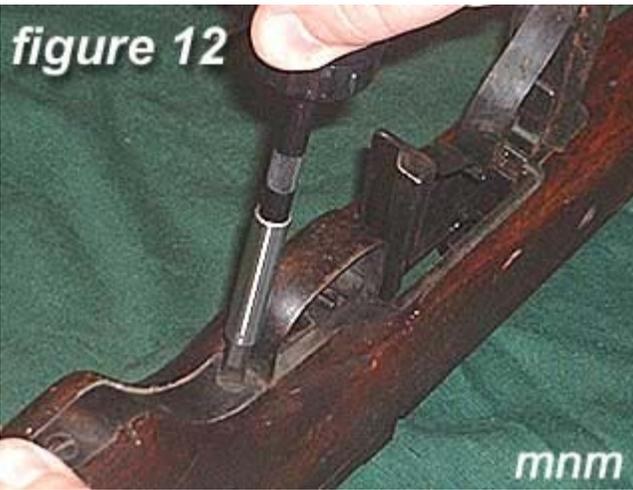
12) Remove the **middle trigger guard screw**.
