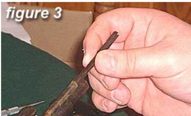
3) Remove the **stacking rod** by unscrewing it.
