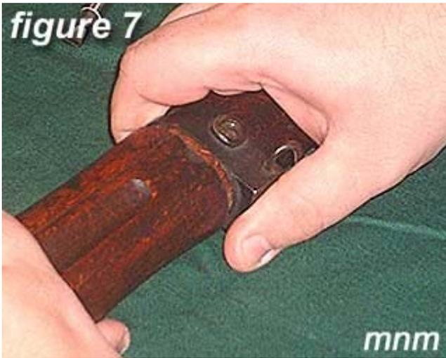
7) Slide the rear barrel band forward.
