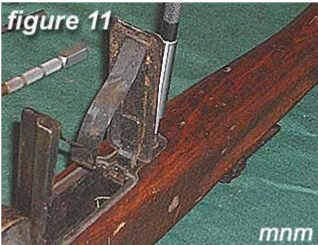
11) Remove the **forward trigger guard screw**.
