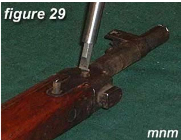
29) Replace forward barrel band screws and tighten.
