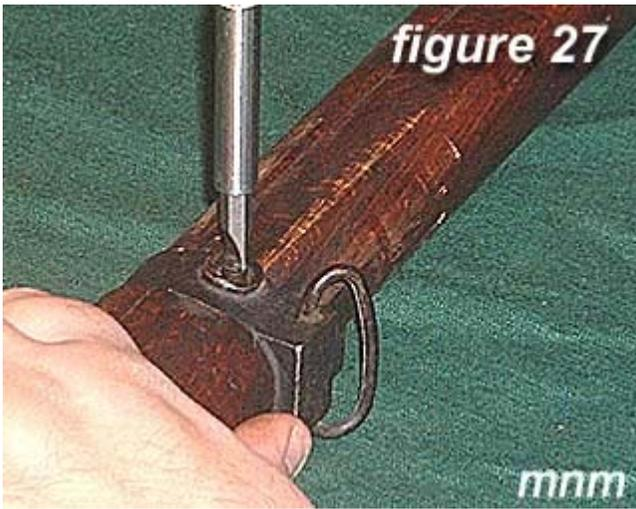
27) Replace the rear barrel band and screw .
