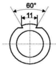
All ANSCHÜTZ rifles have a grooved, 11 mm rail to accept mounts for a telescopic sight.
