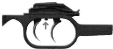
The models of the series 1400 ST and 1500 ST are equipped with a double set hunting trigger. The purpose of this trigger is to fire the shot with a minimum of trigger pressure (hair trigger). The double set trigger is operated as follows:
