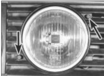
7.4 Foglight beam alignment adjuster screws (arrowed)
