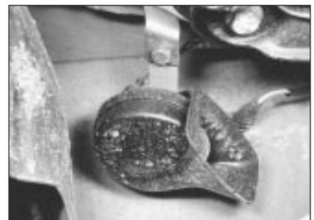
24.1b High tone horn location - twin horn installation
