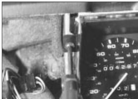
16.3 Instrument panel screw removal
