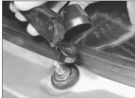
26.3 . . . and withdraw arm from spindle
