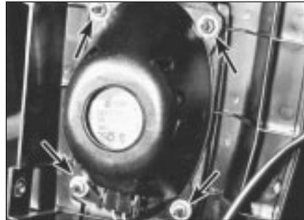
32.5 Luggage compartment loudspeaker retaining nuts (arrowed)
