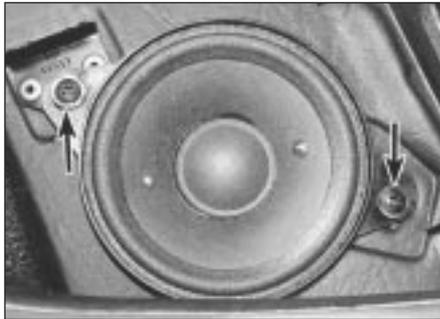
32.3 Facia-mounted loudspeaker retaining screws (arrowed)
