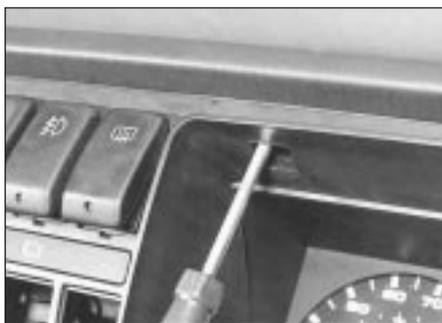
**18.6b** Remove instrument panel retaining screws at top
