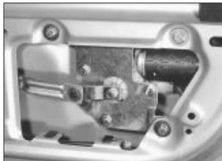
28.4b Rear wiper motor mounting in tailgate
