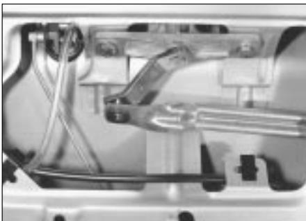
28.4a Rear wiper bearing mounting and connecting rod
