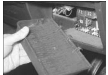
3.1 Removing fuse/relay unit cover
