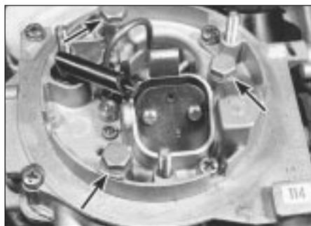
13.8 Carburettor securing bolts (arrowed) - Pierburg/Solex 2E3
