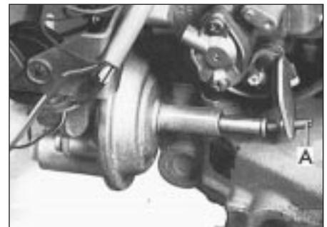
17.39b Fast idle adjustment screw (A)
