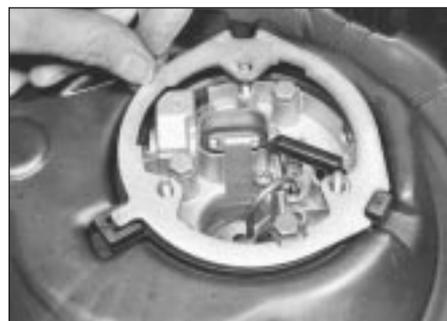
3.2 Removing air cleaner body retaining ring - 1.3 litre
