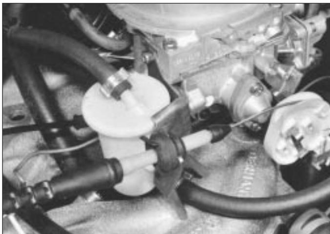
10.3 Accelerator cable to carburettor throttle control
