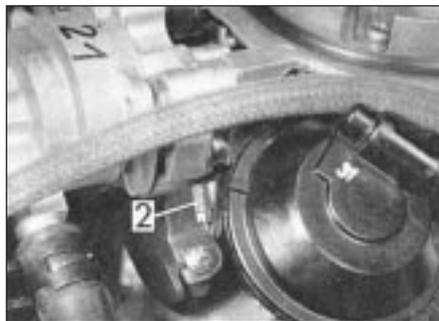
16.10 Fast idle speed adjustment screw (2)
