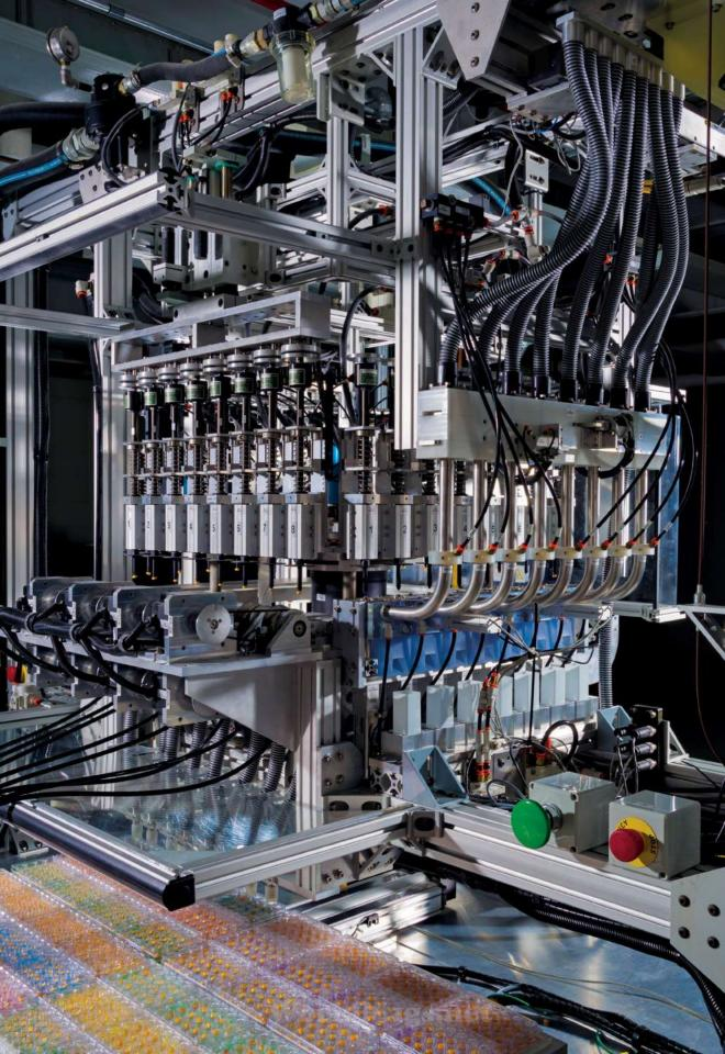
Automating the search for valuable genes, Monsanto's seed chipper cuts tiny samples from thousands of corn kernels a day—without harming the embryonic plant within. Other machines extract and analyze the DNA from each sample. Breeders then plant only the few kernels in a million with the desired trait, such as resistance to pests or drought.
