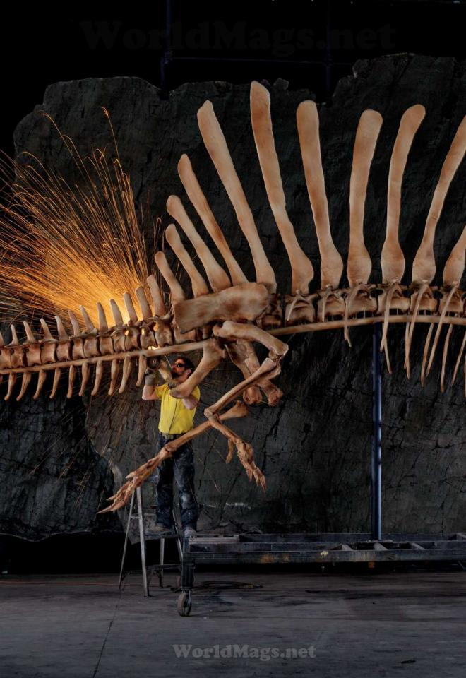
Workers grind the rough edges off an anatomically precise, life-size *Spinosaurus* skeleton created from digital data. Scientists assembled a computer model from CT scans of fossils, images of lost bones, and extrapolations from related creatures, then expressed it in polystyrene, resin, and steel.
