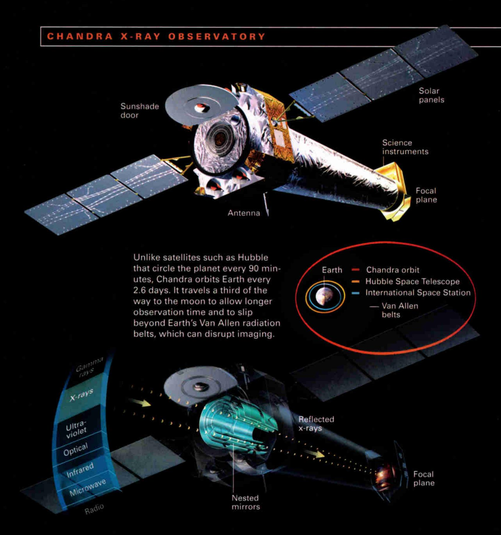
X-rays are photons of light with extremely short wavelengths within the electromagnetic spectrum. They reflect off a mirror only if they graze it at a very low angle, like a stone skipping on water. So Chandra's designers placed four pairs of nested
