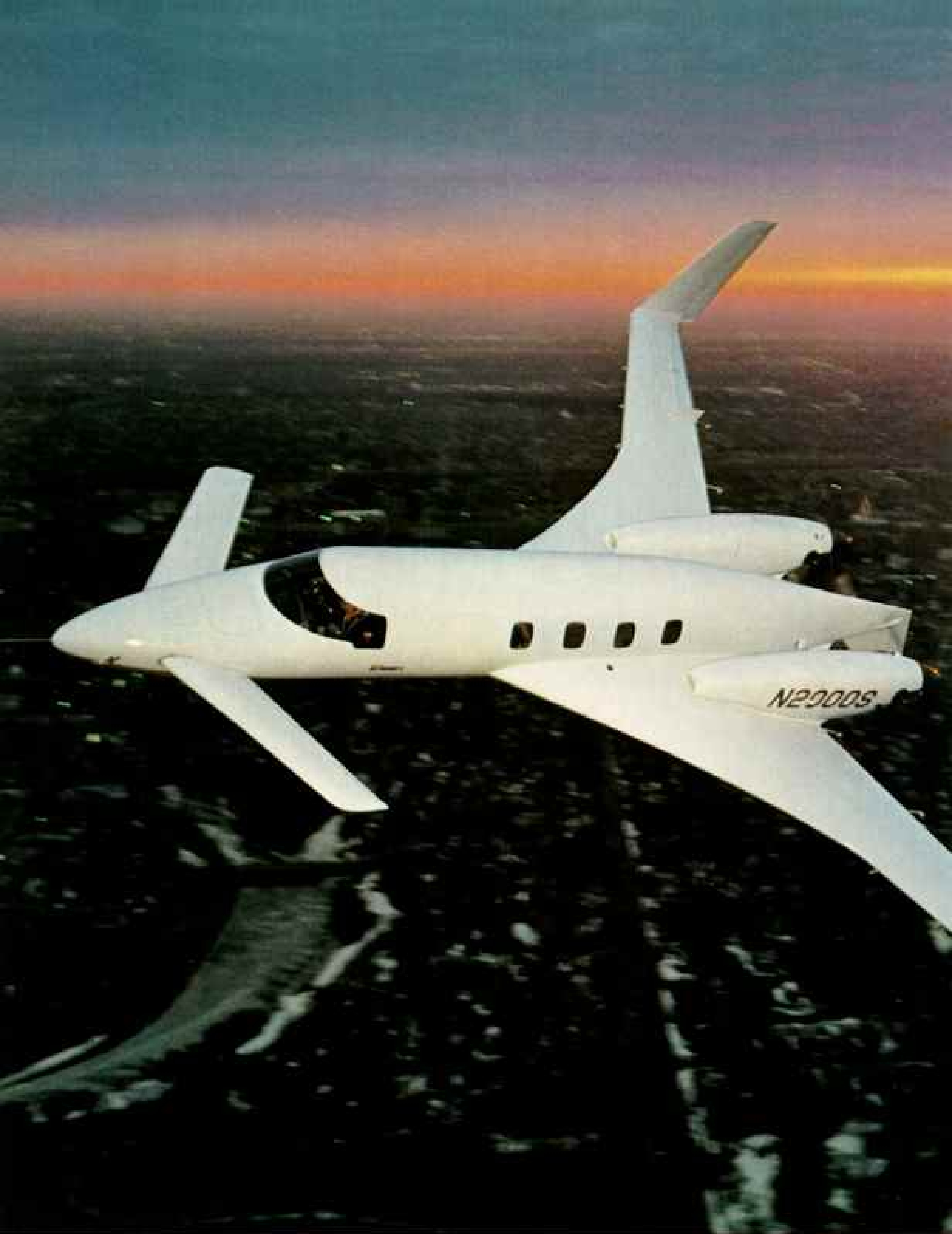
Starship 1, Beech Aircraft's bid to set tomorrow's standard for corporate aviation, sweeps over Wichita. The three-million-dollar aircraft, with small wings at the nose for stability and jetprop engines for fuel economy, will be available in 1987. Also headquarters for
