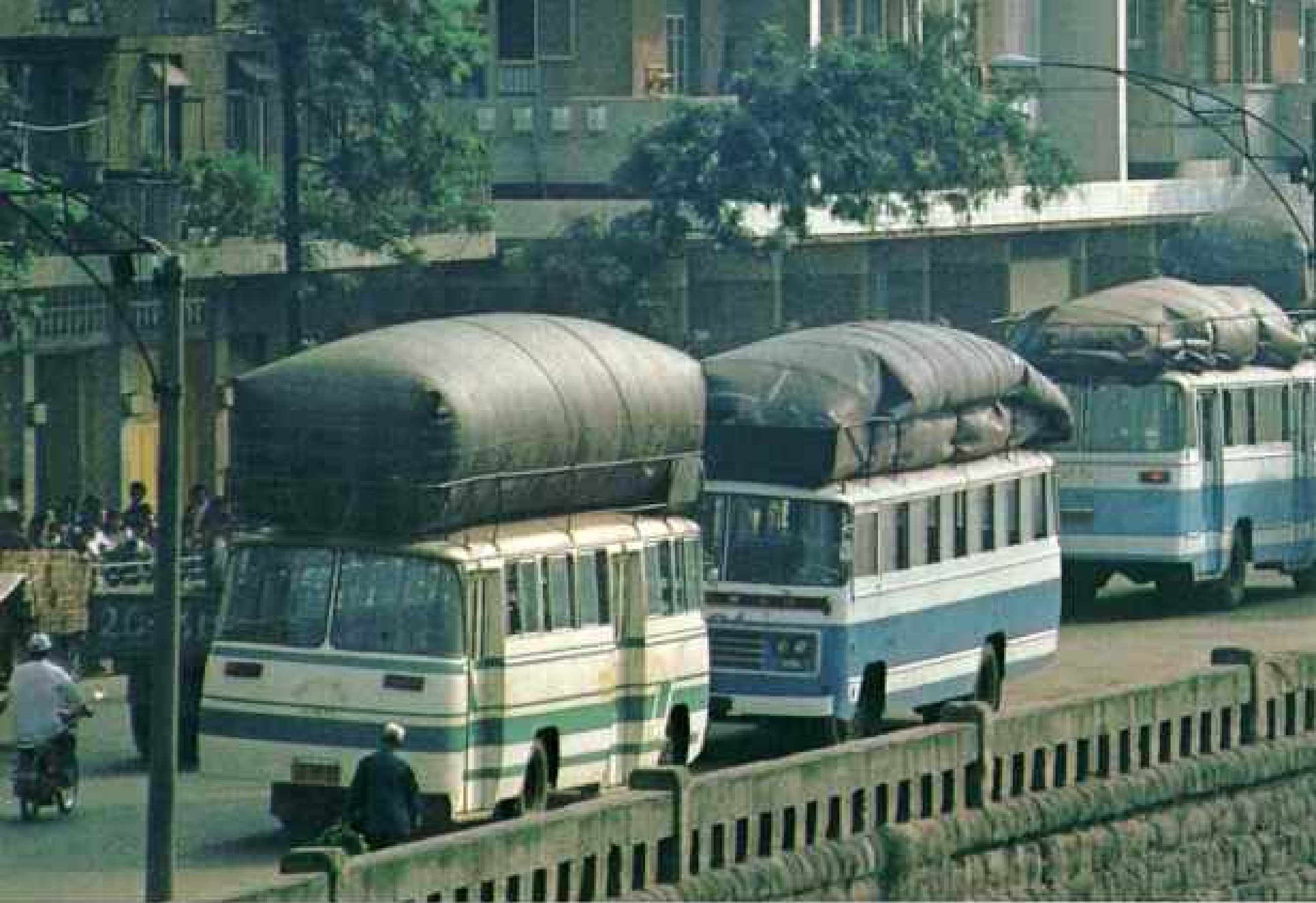
Huffing along with roof bags full of natural gas, commuter buses line Binjiang Road in Zigong. The contents of the 1,000-cubic-foot bag propel the bus for 50 miles
