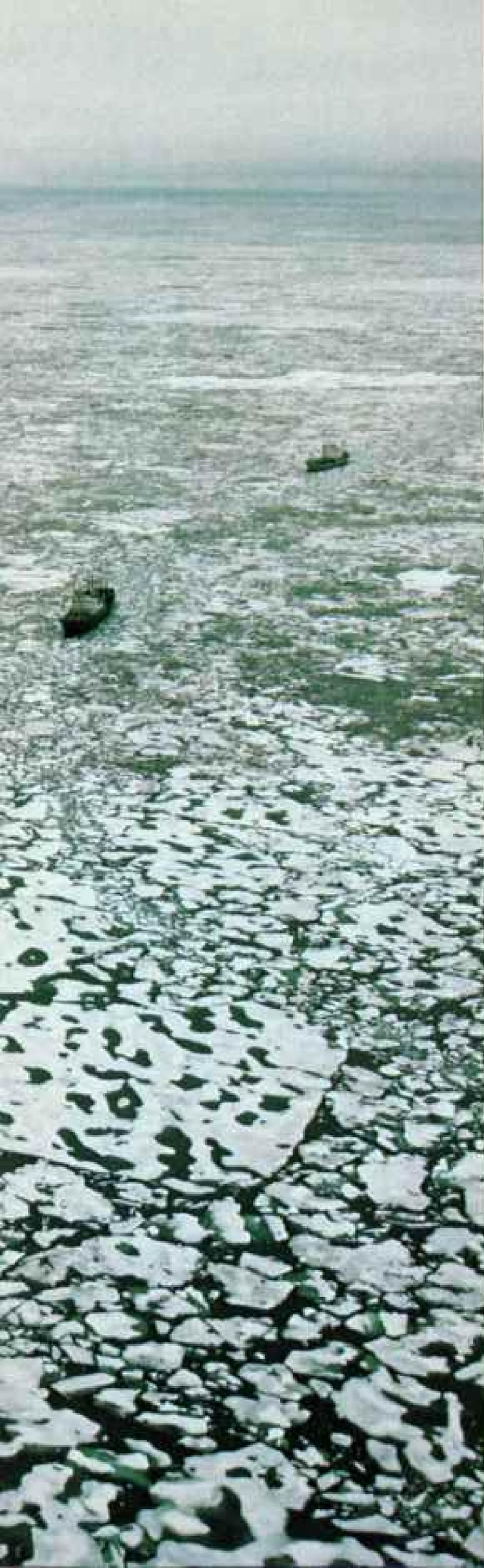
*Wedging through floes nearly five feet thick, Soviet icebreakers lead a freighter convoy along the northern sea route. Despite a Soviet fleet that includes three nuclear-powered icebreakers, ice shuts down shipping from November to March.*
