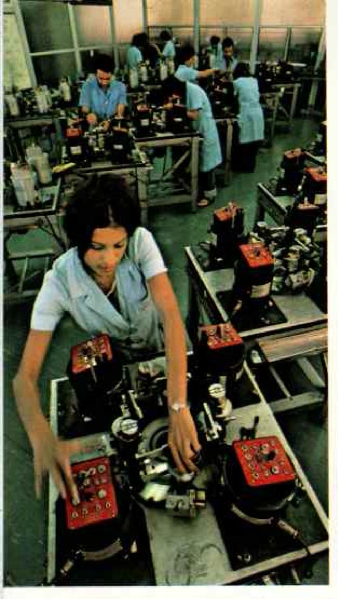
Assembly-line diamond cutting at the Barmatz factory in Tel Aviv (left) sets a hundred automatic polishing machines to work on four stones at a time, turning out about 1,200 eight-point (8/100 of a carat) diamonds a day. The operation helps keep up with a market that has shifted from single large stones to settings of multiple small ones. Israel's largest export, diamonds generate more than a billion dollars a year,
