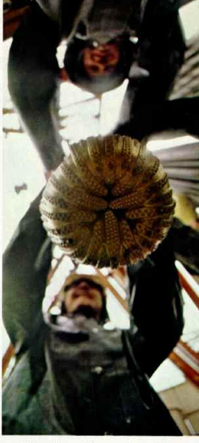
Diamonds aren't forever, at least not in rock-munching oil-rig bits. But they do last many times longer than conventional steel roller bits. Studded with 312 carats of diamonds, this 81/2-inch bit made by Utahbased Christensen Diamond Products, U.S.A., spearheads a search for oil in southern Louisiana.
