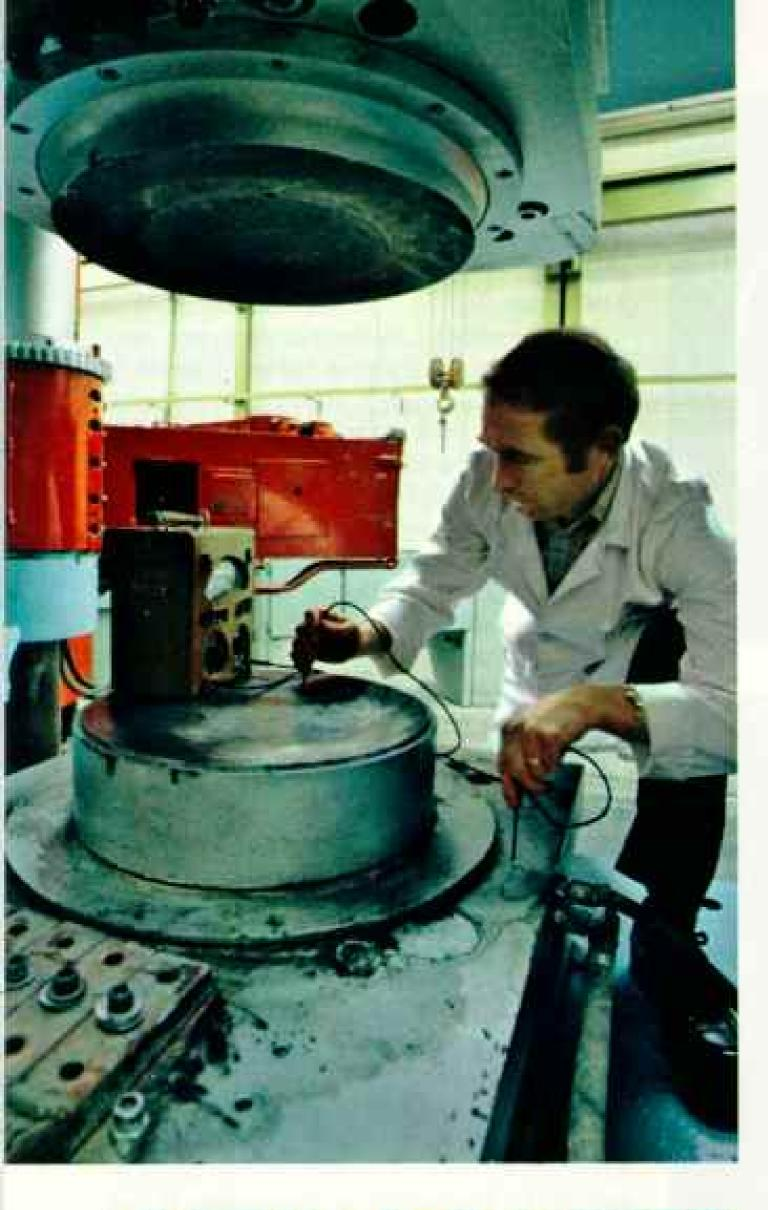
How to make a diamond? Bring pressure of a million pounds per square inch to bear on graphite as the material is heated to 2500° to 3500°F. The result—1/2-mm synthetic diamonds embedded in a matrix (lower left), whose metal acts as a catalyst in the process, pioneered by General
